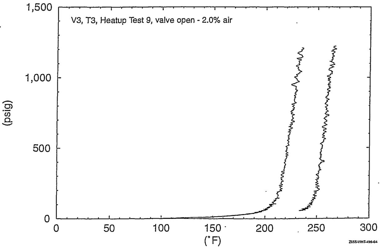
**Figure 8.** Pressure versus temperature with 2.0% entrapped air.
