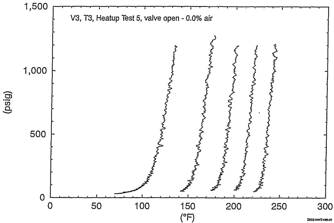
**Figure 5.** Pressure versus temperature with no entrapped air.
