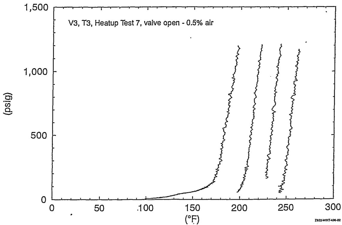
**Figure 6.** Pressure versus temperature with 0.5% entrapped air.
