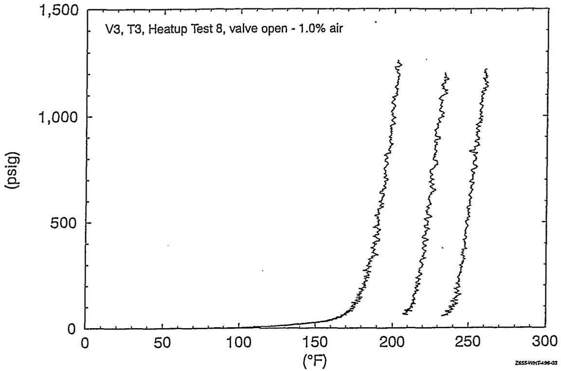
**Figure 7.** Pressure versus temperature with 1.0% entrapped air.
