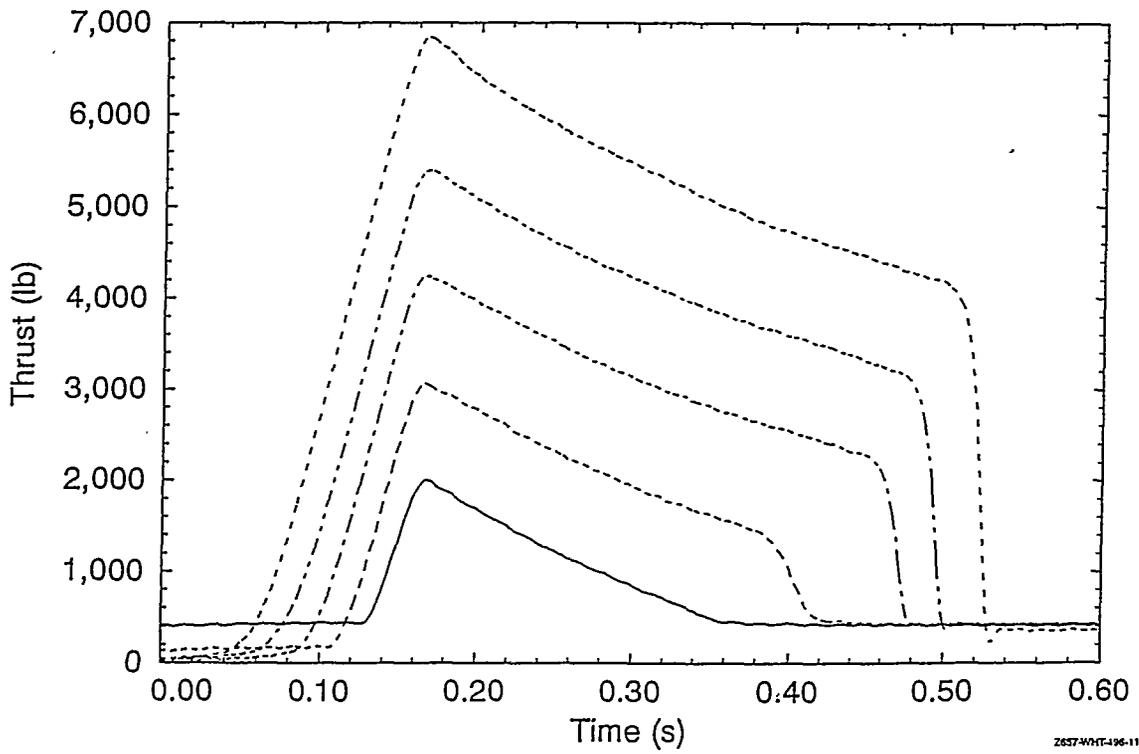
**Figure 4.** Opening thrust measurements from pressure locking tests at five different pressures.
