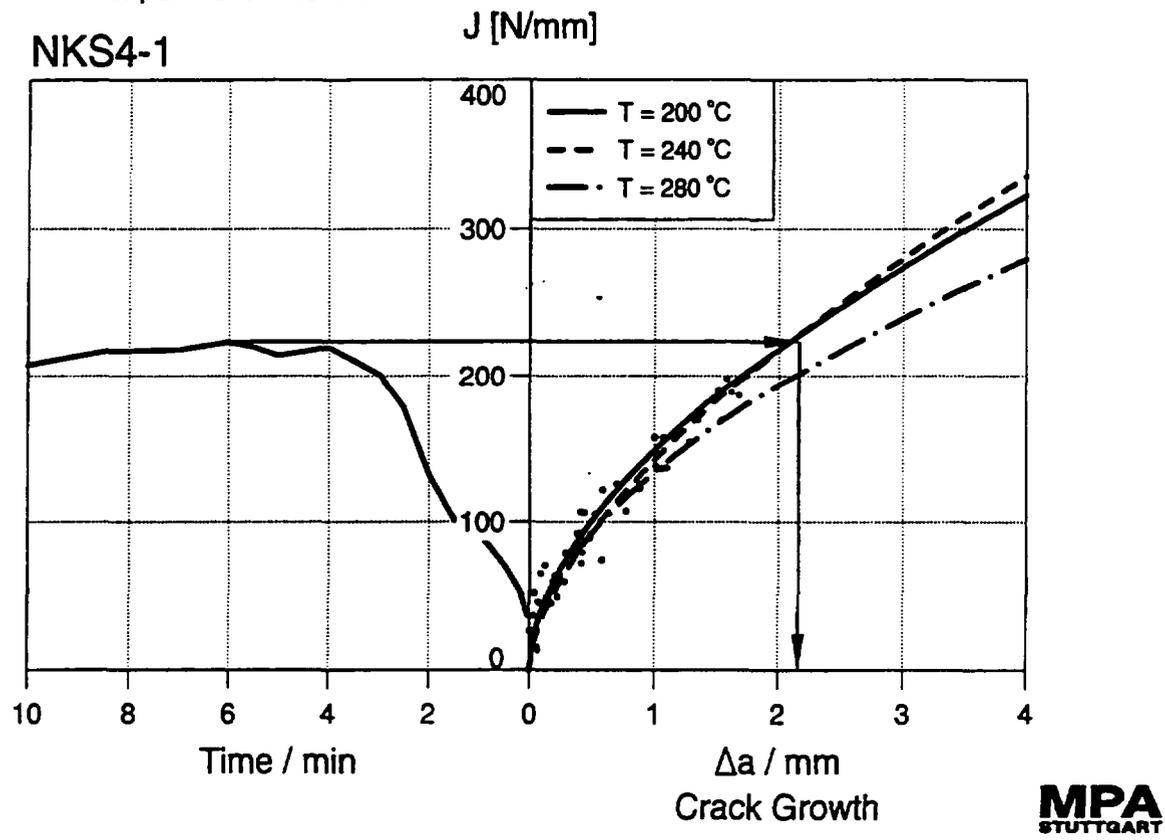
Fig. 6: Procedure to evaluate amount of stable crack extension from load path and crack resistance curve of thermal shock experiment NKS 4-1
