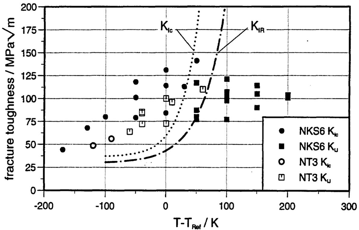
Fig. 8: Fracture toughness data  $K_{Ic}$  and  $K_{IJ}$  normalised to the transition temperature  $T_{ref}$  of the MoV steel of the thermal shock specimens NKS 6 and NT 3
