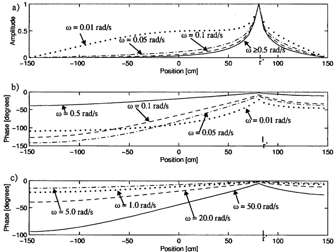
Fig. 1. Space dependence of the amplitude and the phase of the neutron noise in the considered reactor system for several frequencies.
