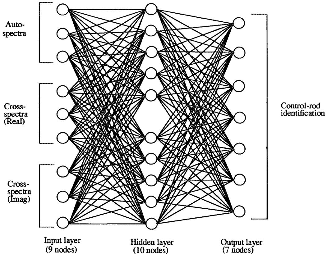
Fig. 3. Structure of the implemented neural network for the case of 3 detectors. For the case of 4 detectors, the input layer consists of 16 nodes instead.
