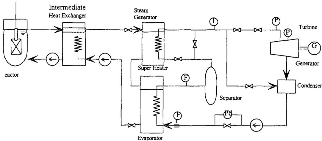
Fig.9 Block Diagram of LMFBR plant Modeled in the Plant Simulator
