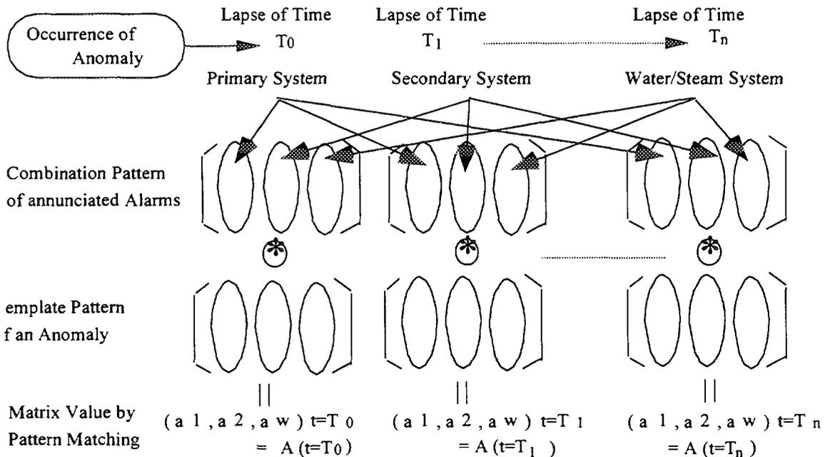
Fig.5 Pattern Matching Method between the Patterns of annunciated Alarms and Template corresponding to an Anomaly using the Changes of Patterns as Time goes by
