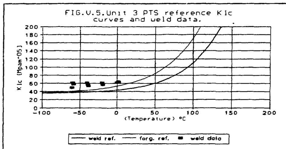
**FIG. 2.** Comparison of the K<sub>1c</sub> reference curves and surveillance results obtained on weldment samples.
