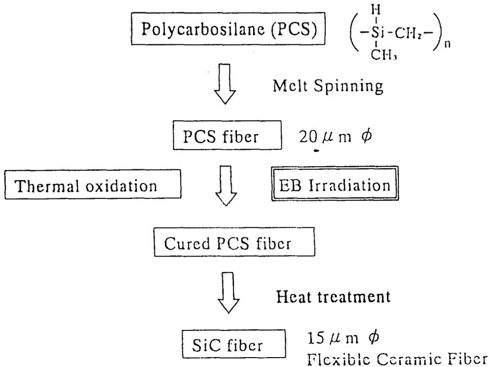
**Fig. 4 Process of SiC Fiber Synthesis from Polycarbosilane**
