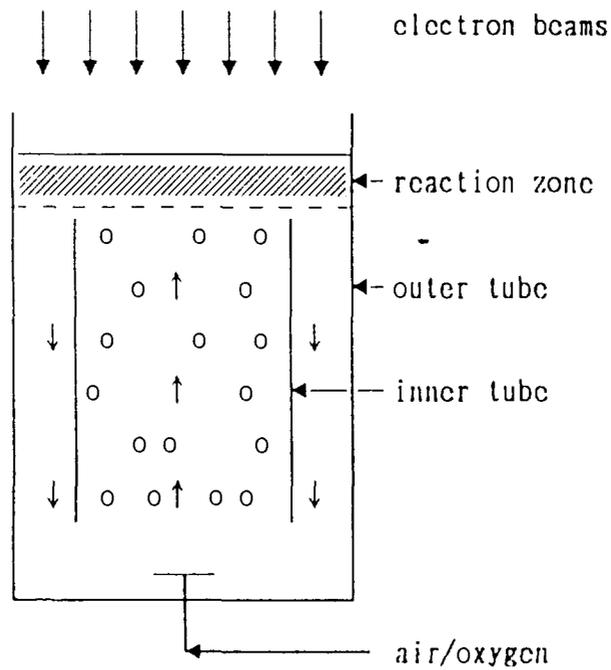
Fig. 2 Dual-Tube Bubbling Column Reactor
