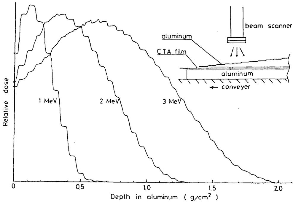
**Fig. 3 Dose Distribution Measurement Using the CTA Tape**
