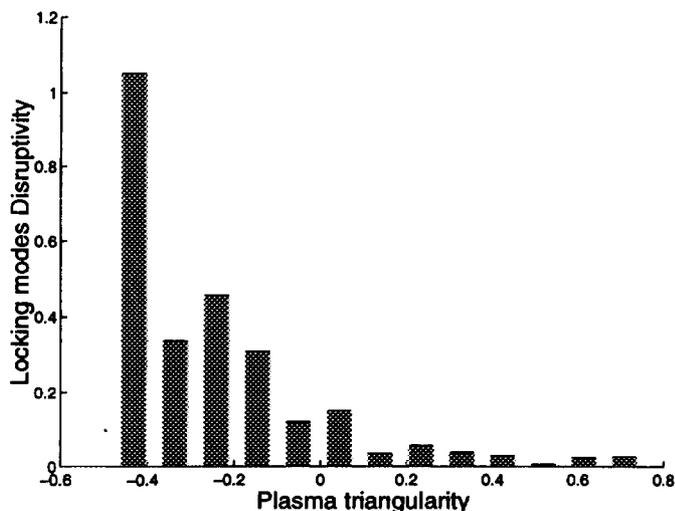
Fig 2: Disruptivity due to locking modes decreases with the triangularity
