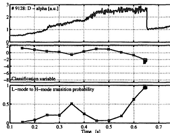
Fig 3:  $D\alpha$  trace shows a L-mode to H-mode transition, the discriminant variable and the associated probability reveals the imminence of the transition by the increase of the transition probability
