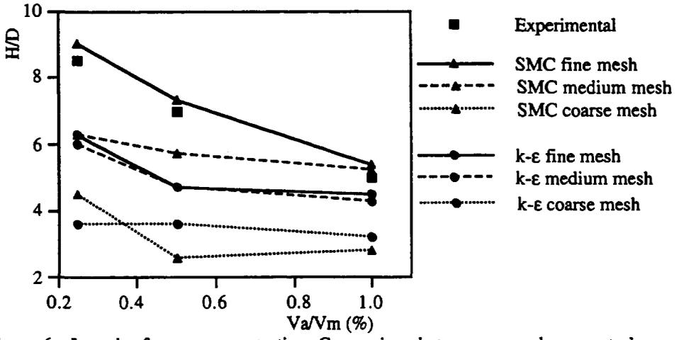
Figure 6 : Length of vortex penetration. Comparison between second moment closure (SMC) and k-ε model. Coarse, medium and fine mesh were used
