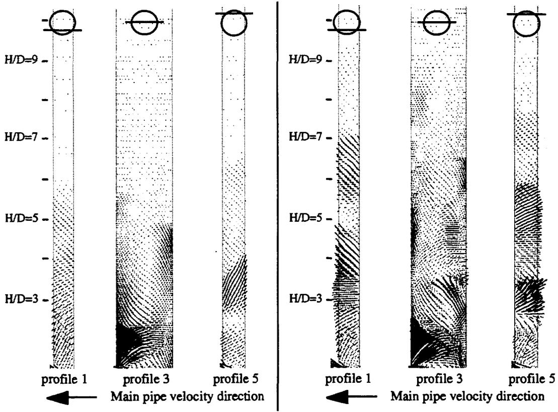
Figure 5 : predicted flow patterns, k-ε model (left) and second moment closure (right). Vector velocities with positive vertical component are displayed in Black and the negative in grey. On the top of the pipe each profile position is shown
