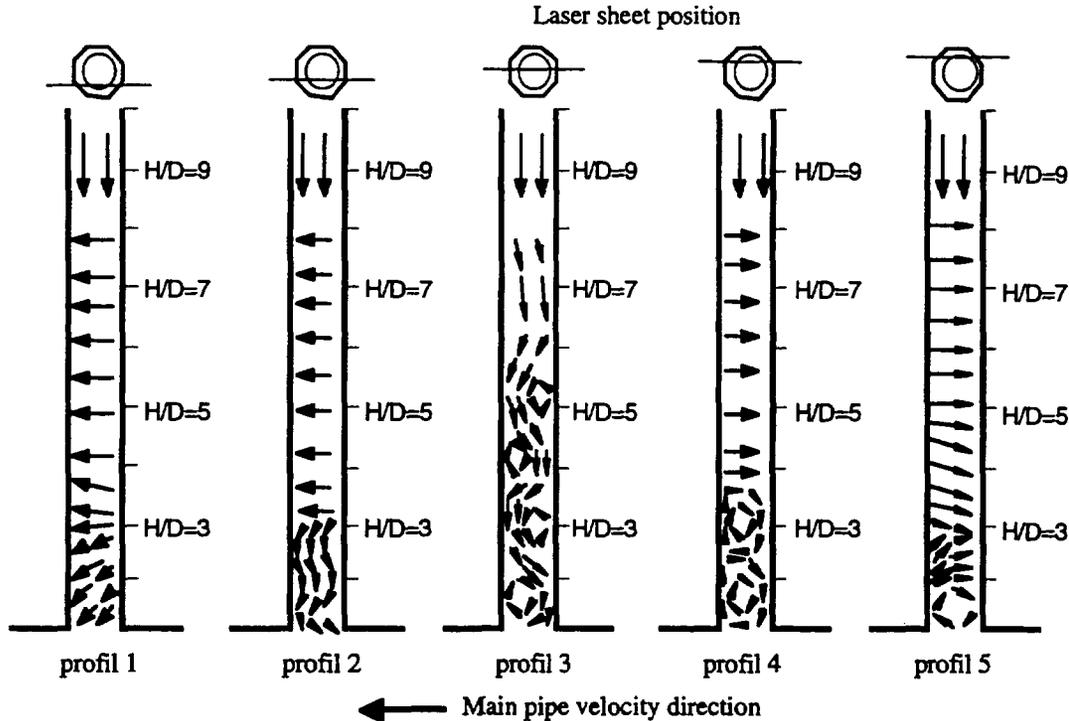
Figure 2 : Sketch of the flow obtained by visualisation ( $V_a = 0.023$ ).
