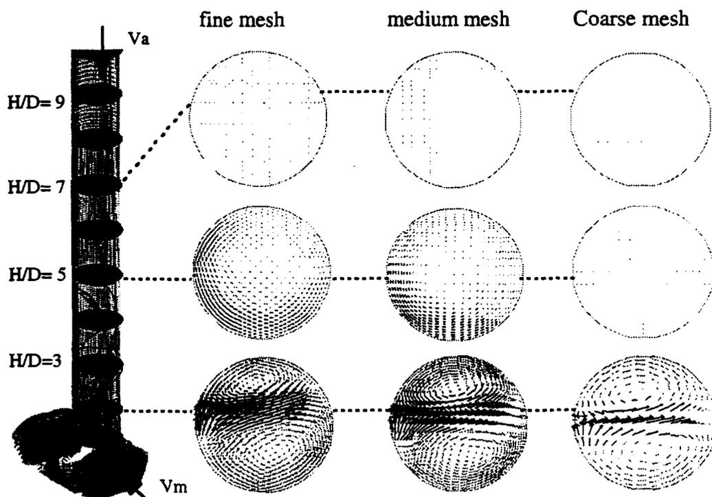
Figure 4 :  $k-\epsilon$  prediction of vortex penetration in the dead leg:  $V_a/V_m = 0.25 \%$ . The legend is the same as figure 2.
