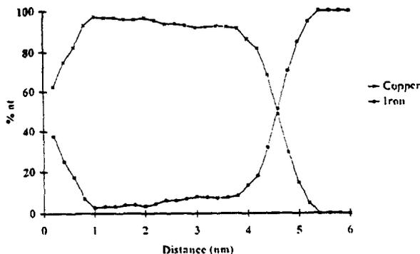
Fig. 2. Iron and copper concentration profiles through the copper particle displayed in Fig. 1.
