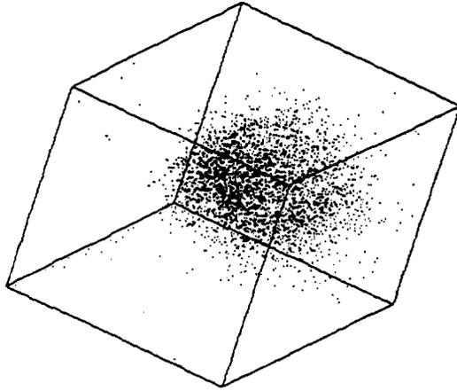
Fig. 1. 3D reconstruction showing the presence of a copper-rich particle in a thermally aged Fe-0.7 wt% Cu alloy (70 h at 500°C). Only a portion of the analyzed volume is represented here ( $6 \times 6 \times 10 \text{ nm}^3$ ). Each elemental dot represents a single copper atom.
