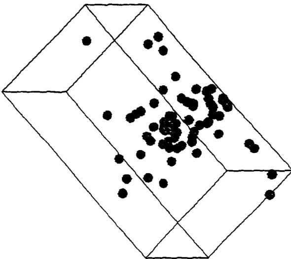
Fig. 6. Spatial distribution of copper atoms in a neutron irradiated Fe-0.1 wt% Cu alloy. The dimensions of the represented volume are  $3 \times 2.5 \times 5 \text{ nm}^3$ . Each grey circle is a single copper atom, black reinforcements give an idea of the local density inside the cluster.
