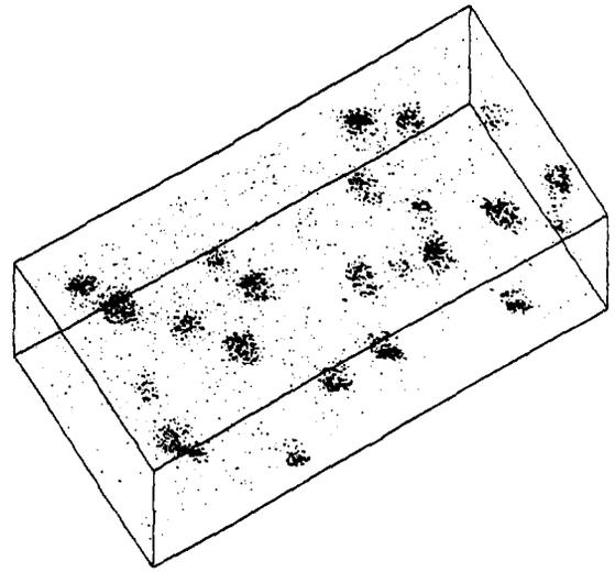
Fig. 3. Spatial distribution of copper atoms in a neutron irradiated Fe-1.4 wt% Cu alloy. The dimensions of the analyzed volume are  $15 \times 15 \times 30 \text{ nm}^3$ . About 23 clusters can be distinguished.
