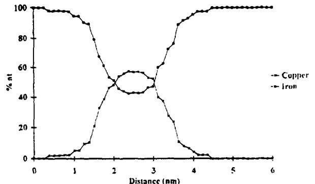
Fig. 4. Iron and copper concentration profiles through one of the clusters displayed in Fig. 3.
