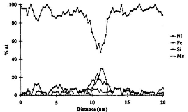
Fig. 8. Iron, silicon, nickel and manganese concentration profiles related to one of the clusters displayed in Fig. 7. Note the rather diffuse aspect of interfaces.
