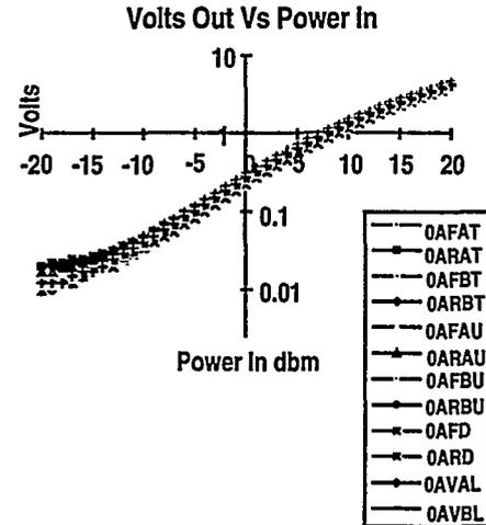
Fig. 4. Amplitude detector voltage out vs. power in.
