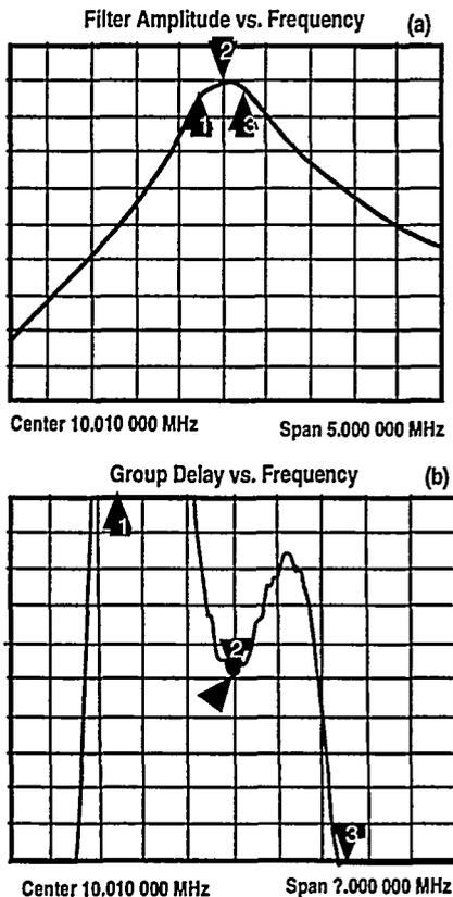
Fig. 3. IF filter amplitude and group delay.
