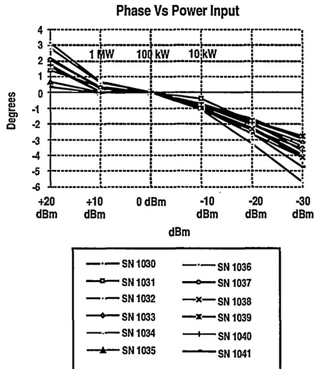
Fig. 5. phase detector accuracy vs input level.
