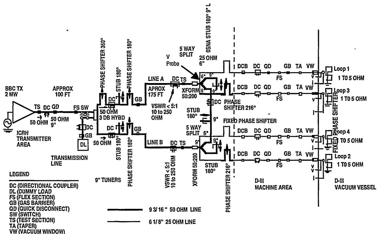
Fig. 1. DIII-D transmission line and antenna tuners
