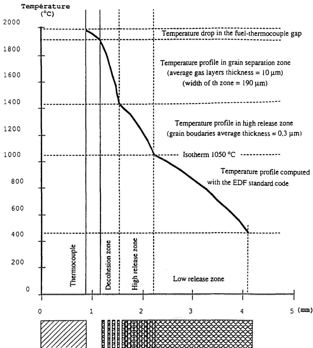
FIG. 3. Radial Profile in the Fuel Pellet
