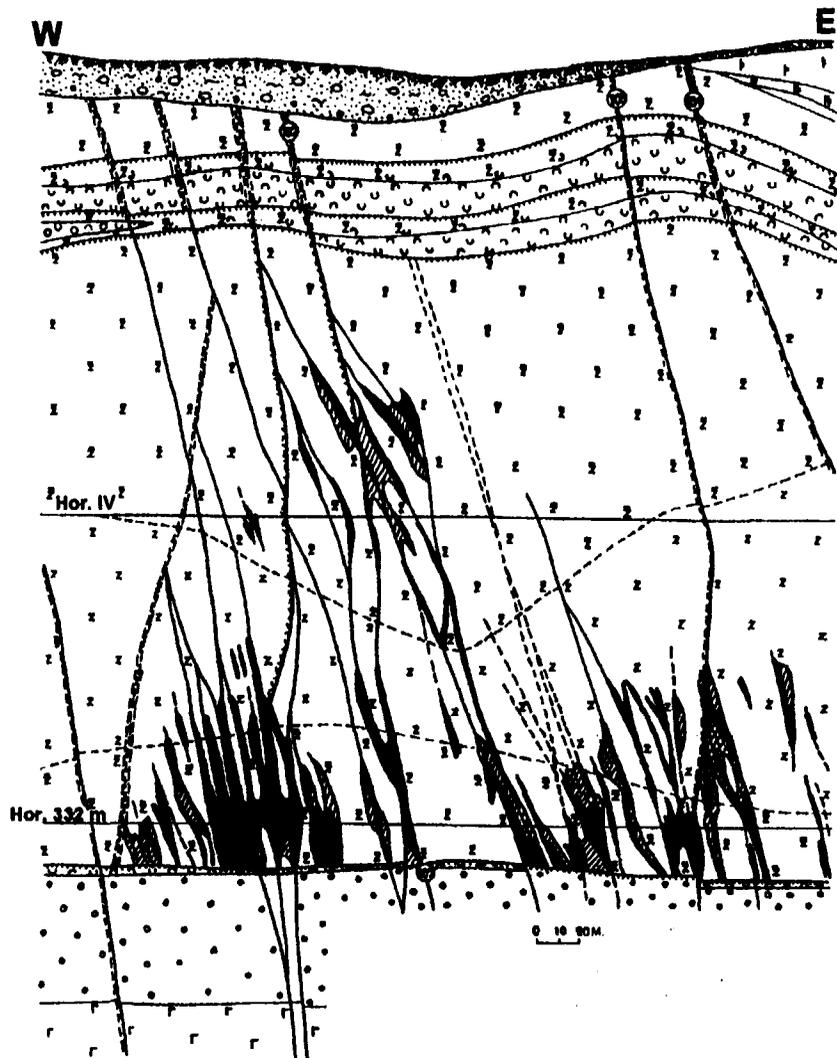
Fig. 4. The Glubiny area of the Streltsovskoye deposit. Geological section on the 97-th prospecting line. Legend see on Fig. 1.
