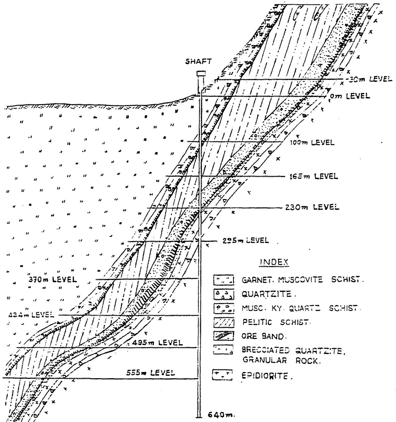
FIG. 3. Transverse section across Jaduguda Hill. Scale: 1:4000.
