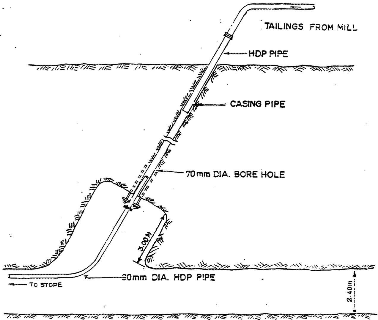
FIG. 11. Sand stowing borehole.
