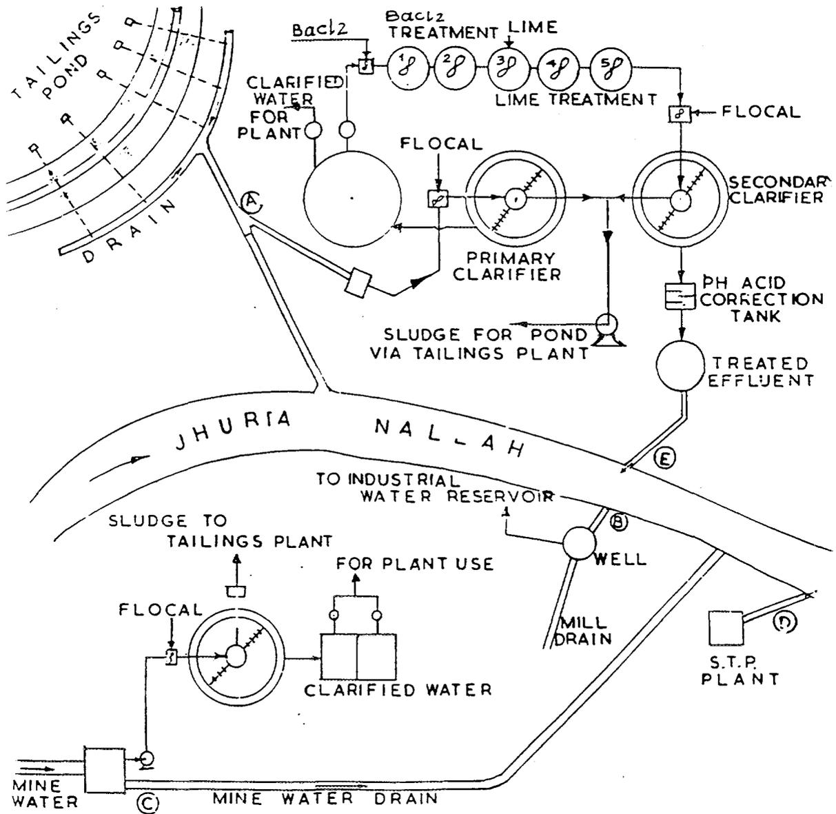
FIG. 17. Flowsheet of effluent treatment plant
