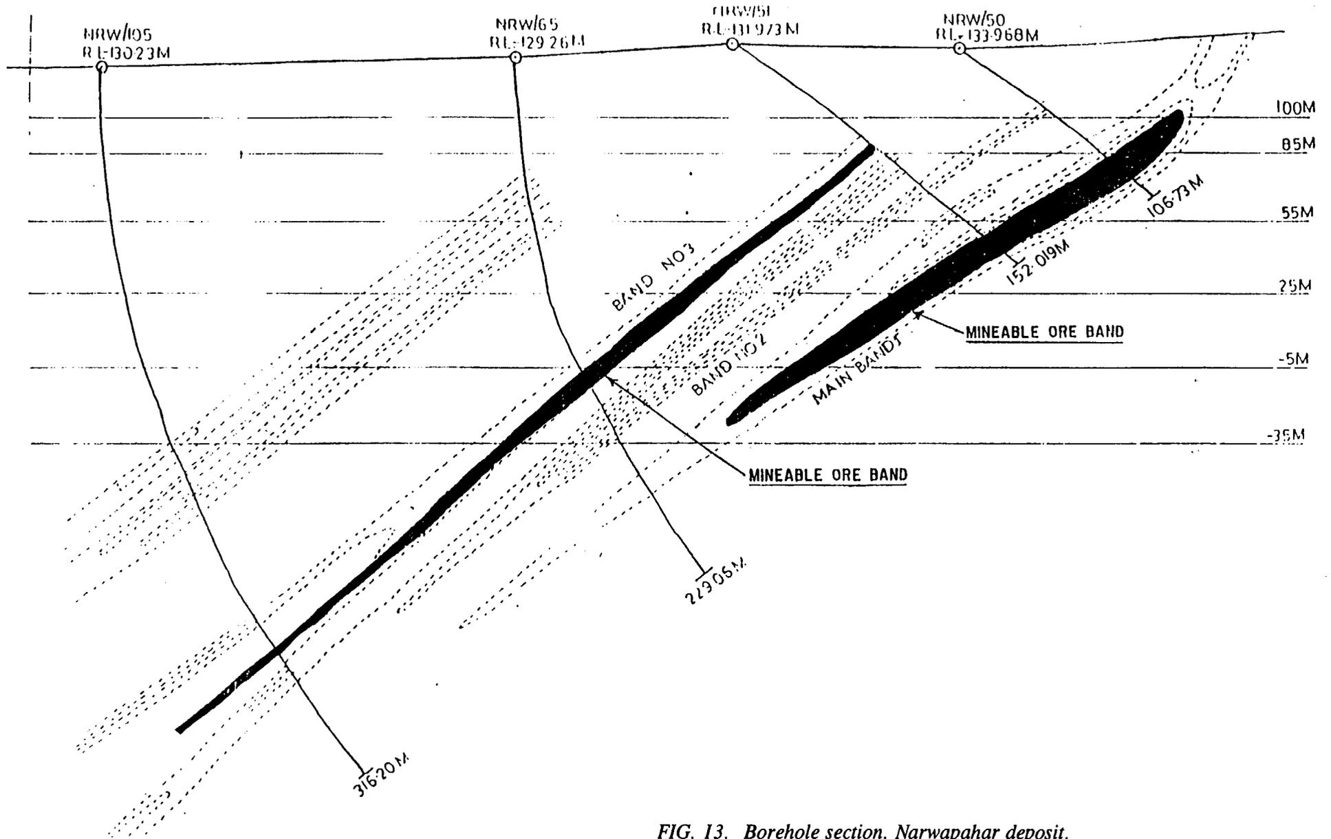
FIG. 13. Borehole section, Narwapahar deposit.
