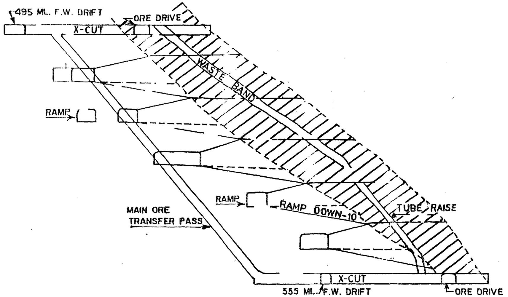
FIG. 8. Transverse section showing the general arrangement of HCF stopping.
