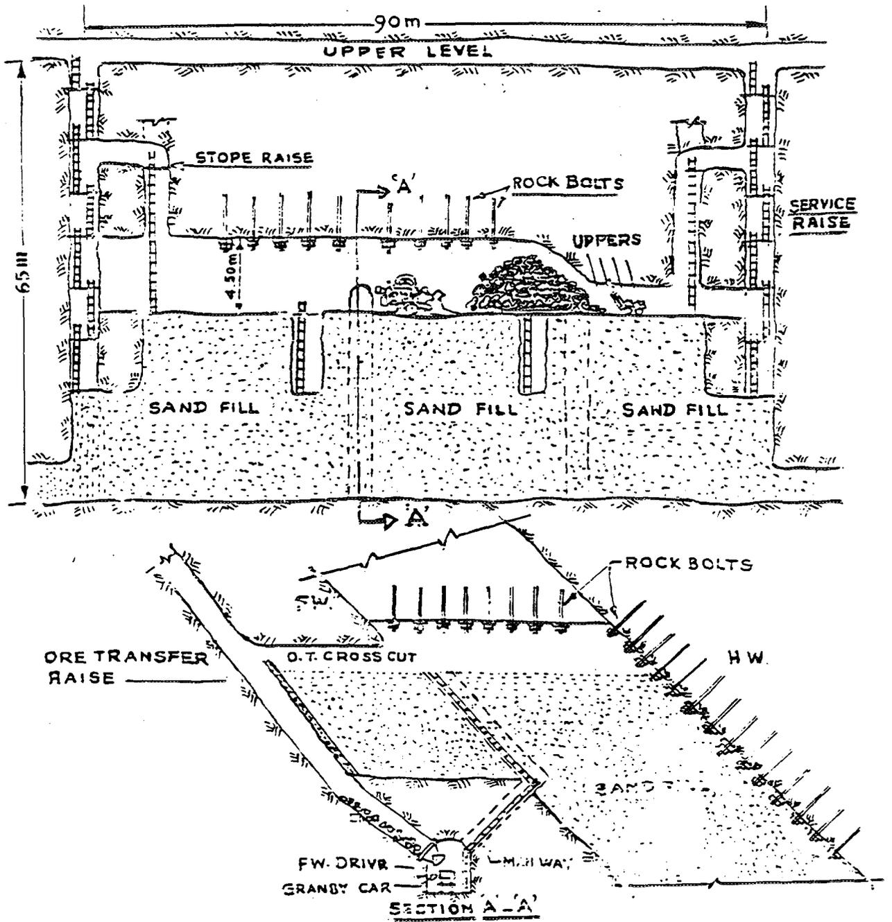
FIG. 6. Cut and fill stope at Jaduguda.
