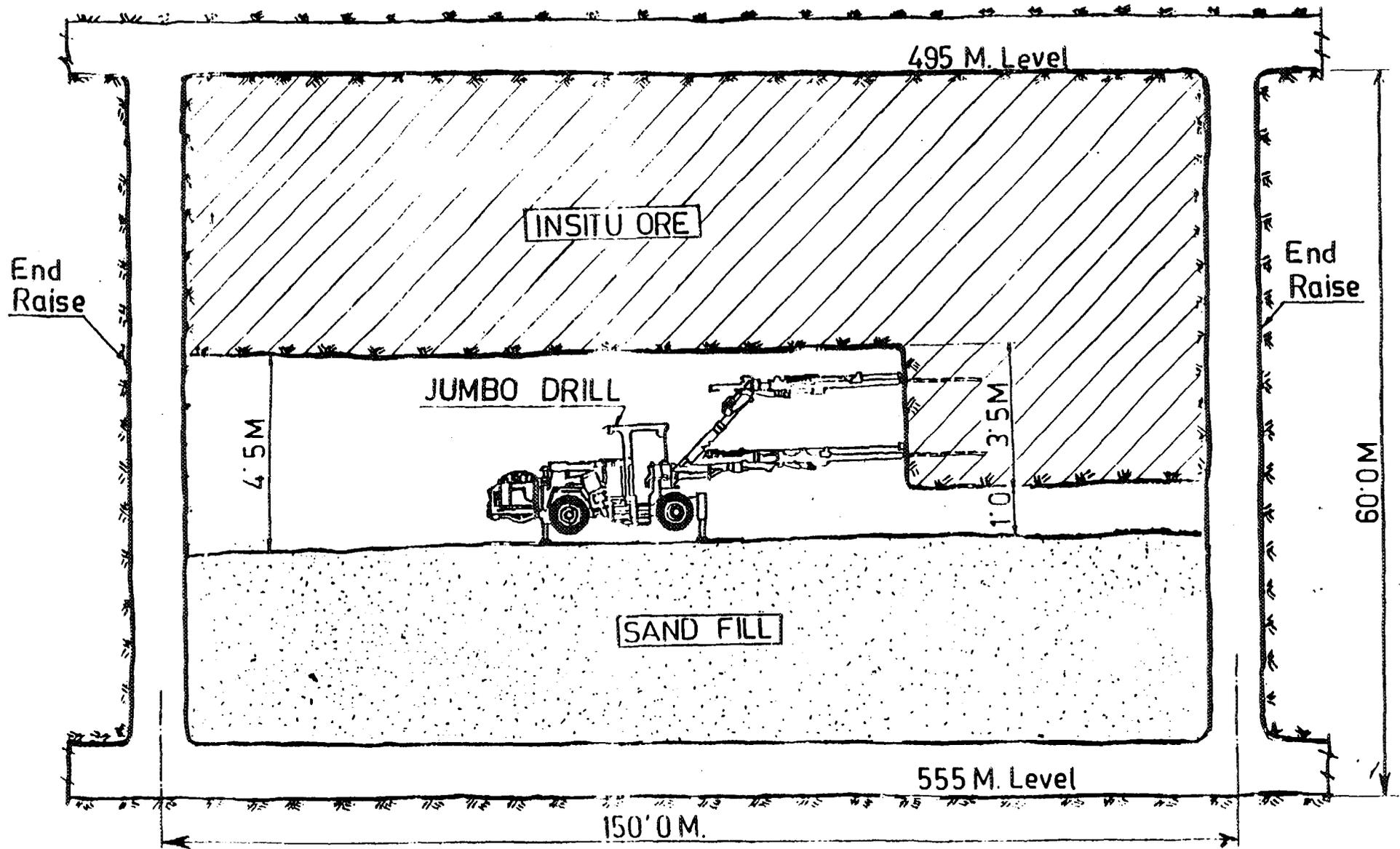
FIG. 7. Vertical longitudinal section; mechanized EO-W5 stope.
