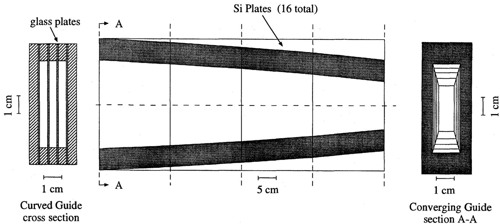
Fig. 2. The converging neutron guide (center and right panels). The NiC-Ti supermirror layers coat all reflecting surfaces of the 16 Si single-crystal plates. A cross section of the curved neutron guide is shown for comparison.
