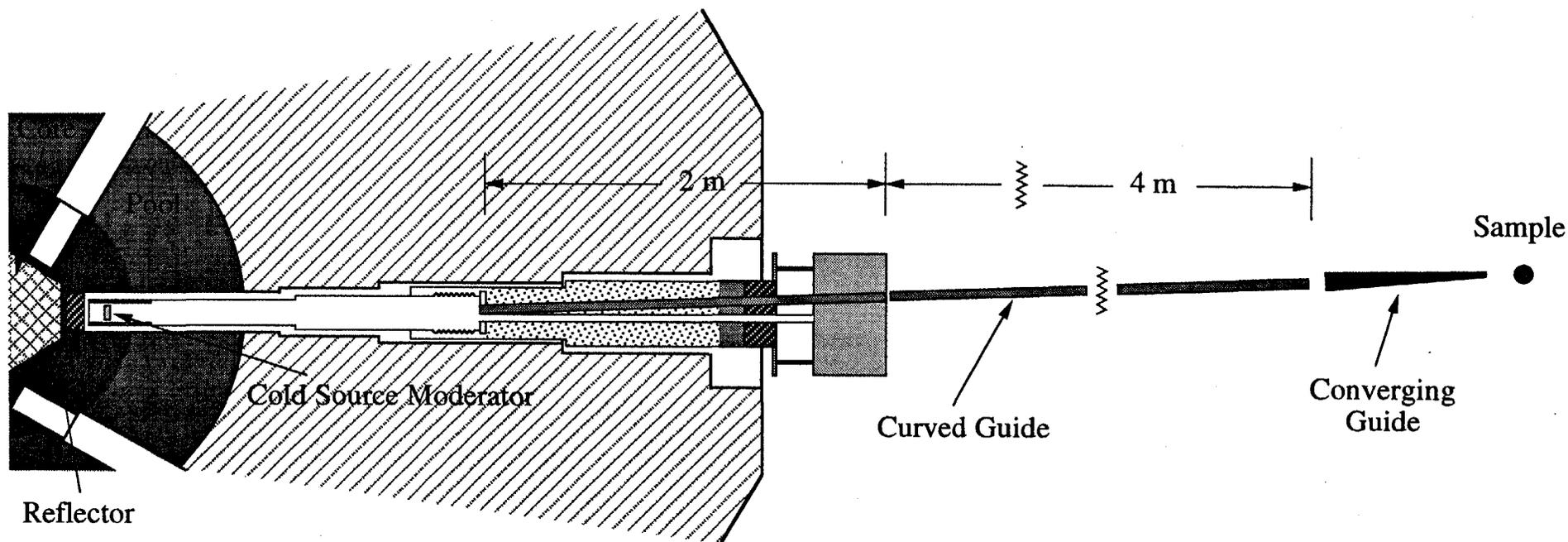
Fig. 1. Cross sectional view of the Texas Cold Neutron Source in the piercing beam port of the UT-TRIGA research reactor showing the location of the 6-m long curved neutron guide and the 80-cm long converging neutron guide.
