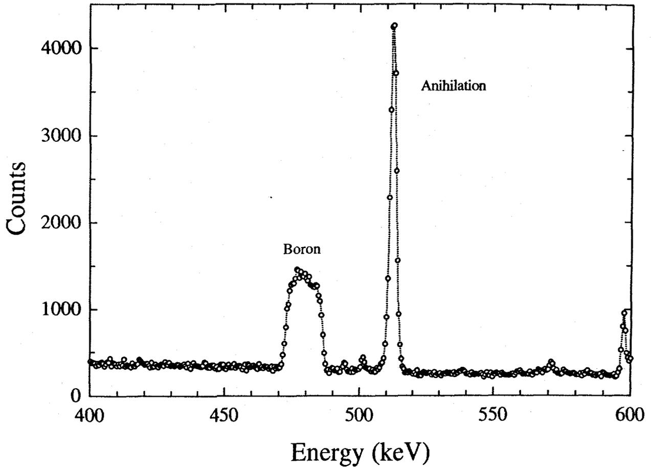
Fig. 6. A segment of the gamma-ray spectrum showing the boron-10 peak for a  $3.8 \mu\text{g}$  sample. The results were obtained by the present, nonoptimized PGAA system with no cold moderator in the TCNS (empty chamber). In this situation, the curved neutron guide selects subthermal neutrons with an average speed of about 1500 m/s.
