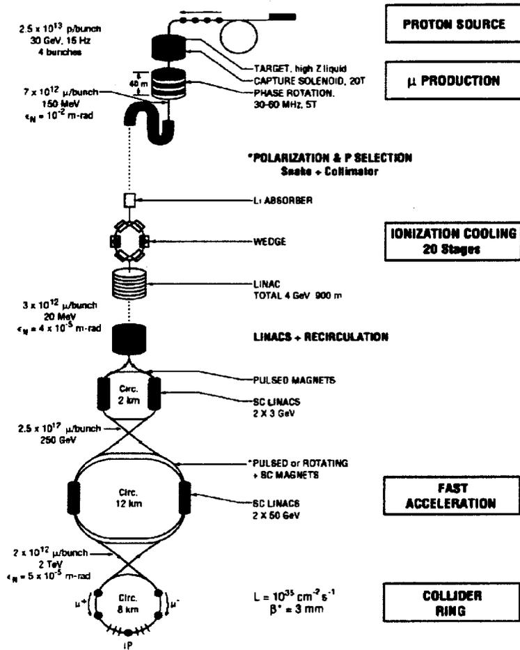
Figure 5: Overview of a 4 TeV Muon Collider
