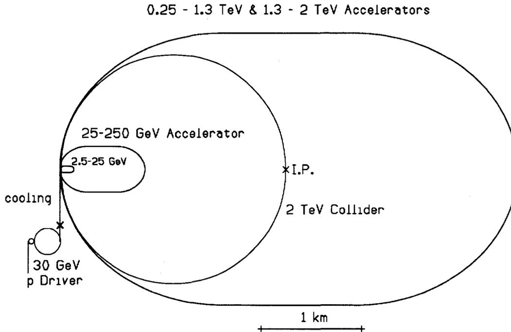
Figure 6: Layout of the collider and accelerator rings.
