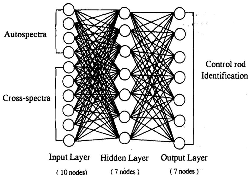
**Figure 1. Structure of the implemented neural network**
