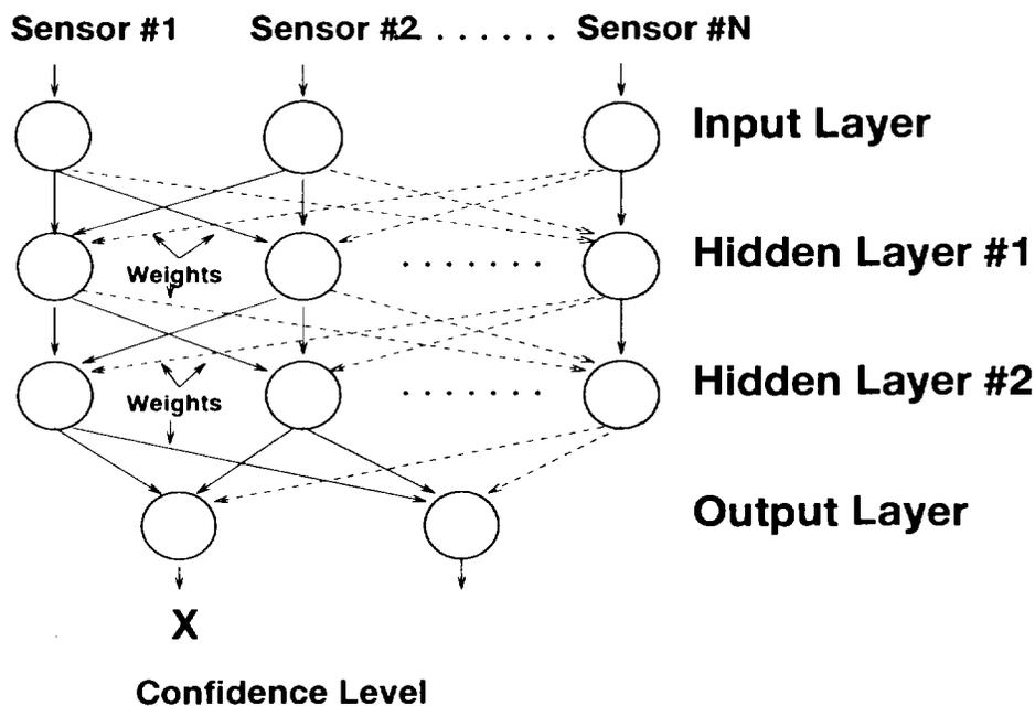
Figure 3: Architecture of a feedforward perceptron network.
