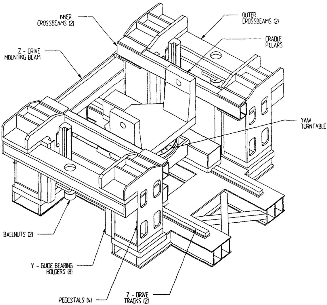
FIGURE 3 ELEVATOR COMPONENTS
