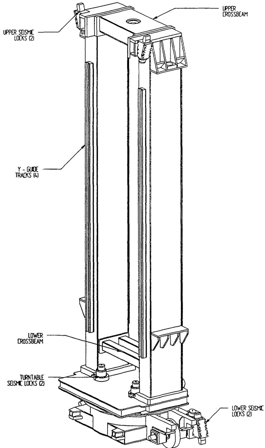
FIGURE 2 CARRIAGE COMPONENTS
