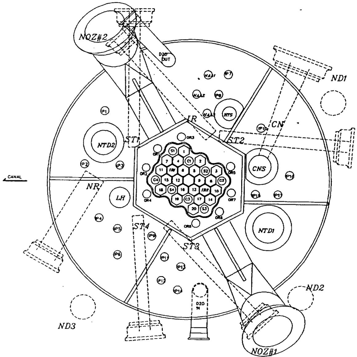
Fig. 2 Plane view of Irradiation Holes and Beam Tubes
