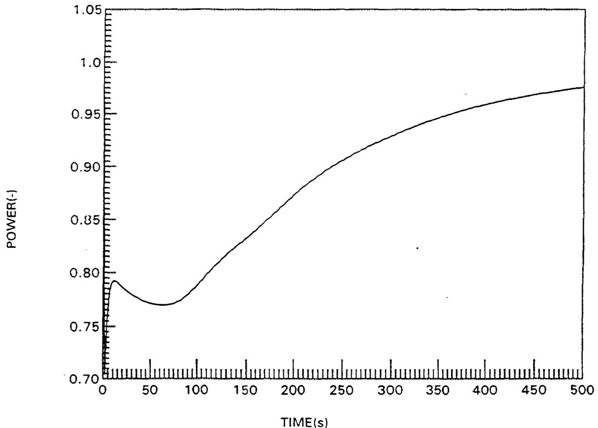
Fig.8 0.5% control rod drop accident:
