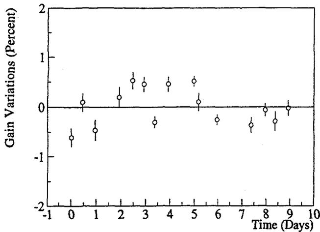
Fig. 5 Gain stability. The percentage change in the gain averaged over several channels, relative to the gain averaged over the entire 9-day running period. The error bars give the one sigma standard deviation.
