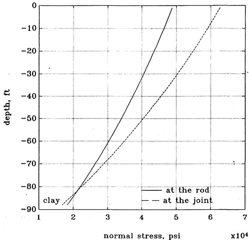
Figure 11. Simulated maximum normal stress.
