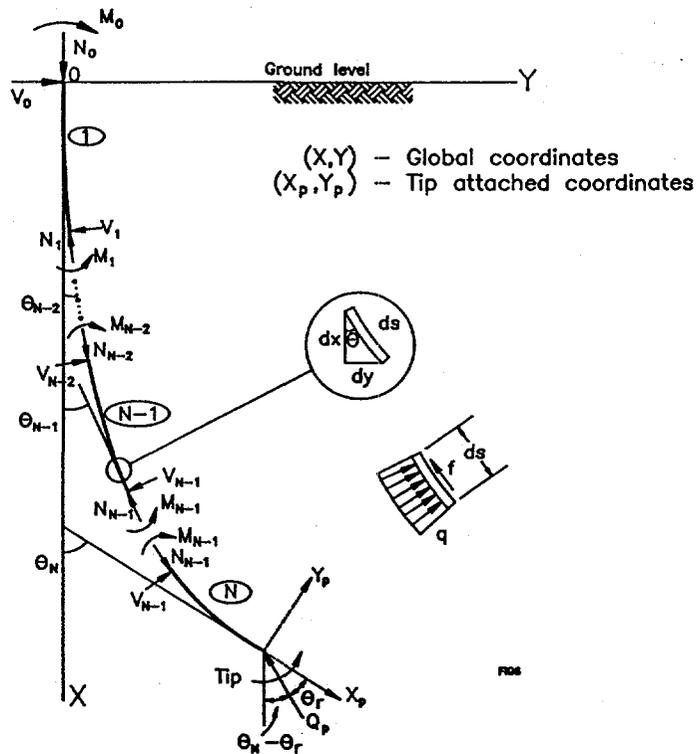
Figure A.1. Penetrometer rod simulation model
