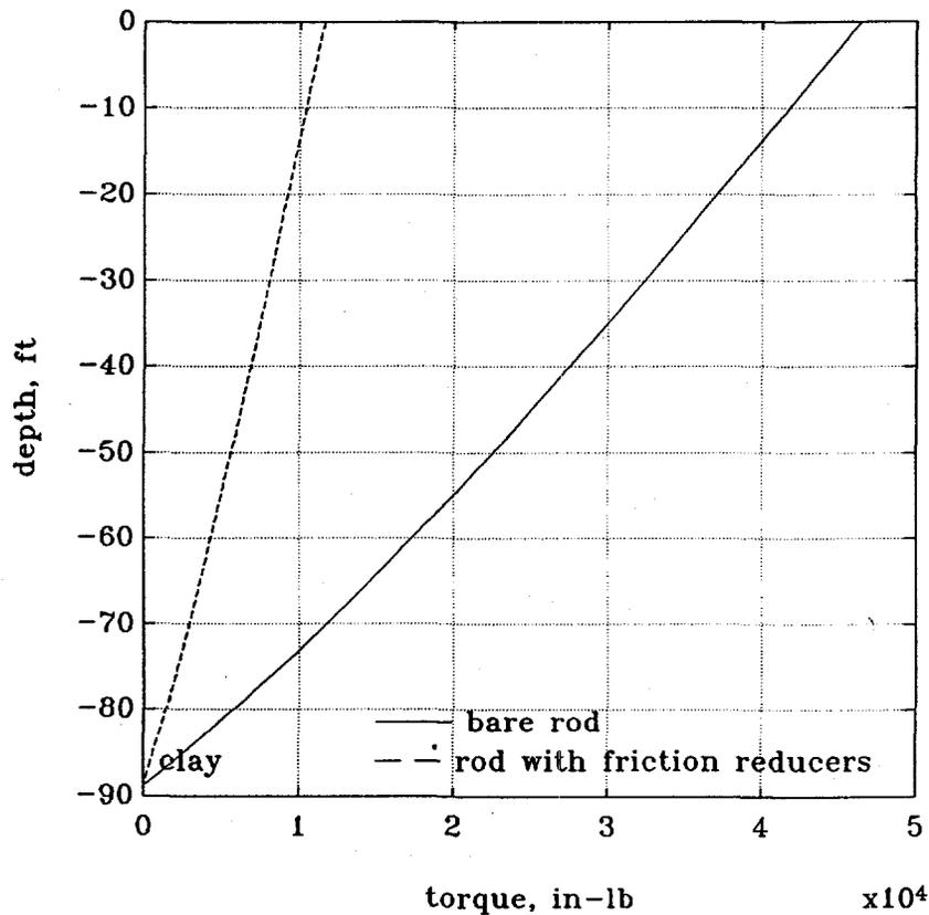
Figure 12. Simulated torque distribution.
