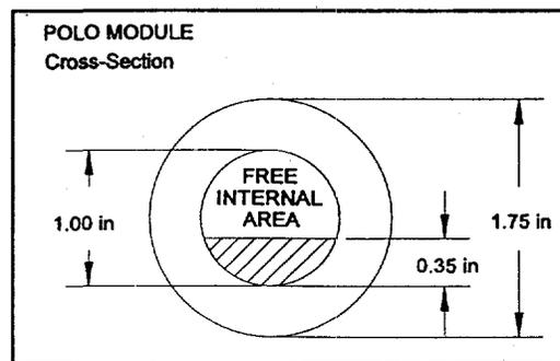
Figure 19. DAQ capsule inside the POLO rod (cross hatched).
