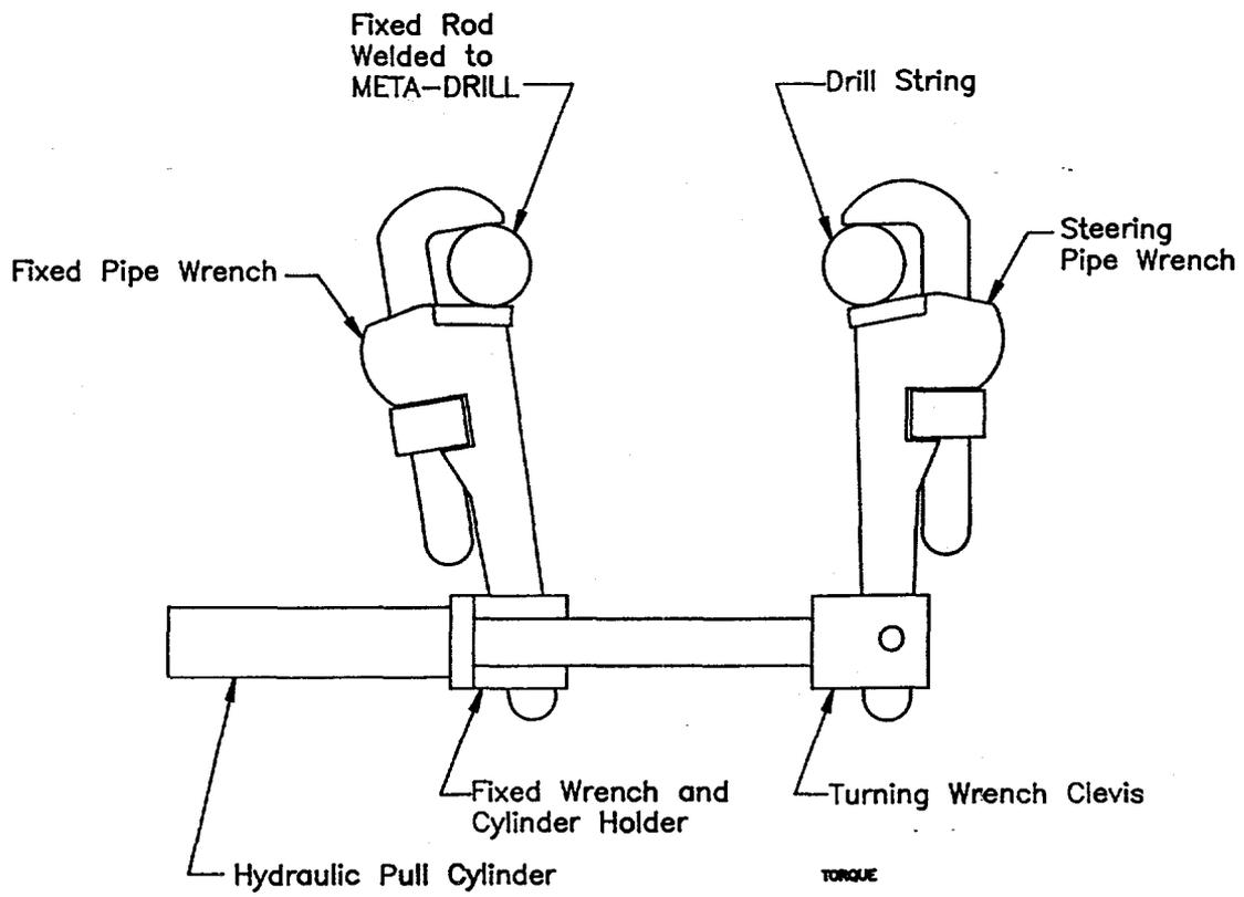
Figure 17. Steering torque mechanism.
