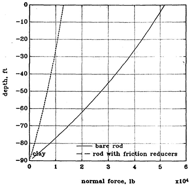
Figure 9. Simulated normal-axial force distribution.
