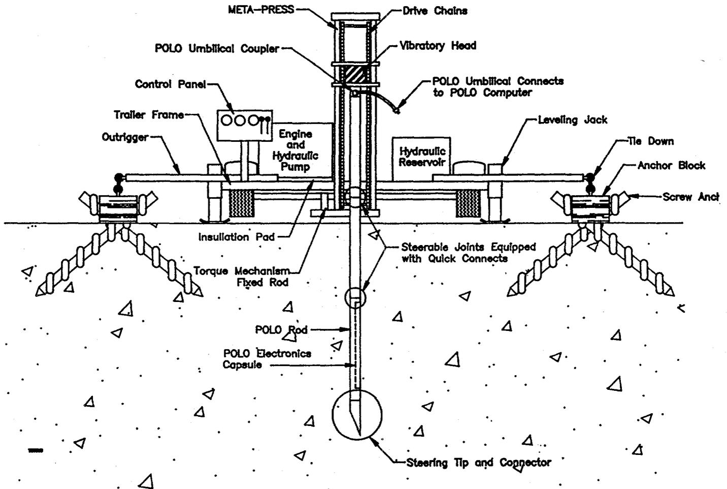
Figure 18. Integrated full-scale penetrometer delivery system.
