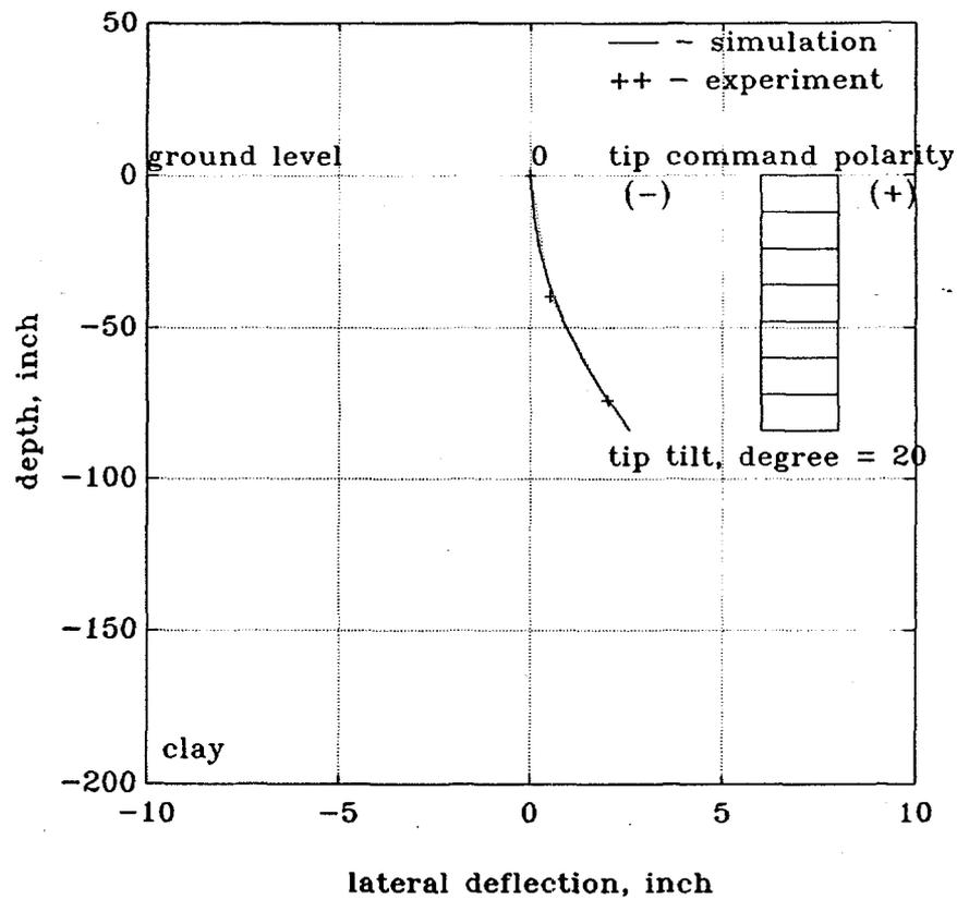
Figure A.2. Penetrometer rod trajectory - comparison between simulation results and test data.
