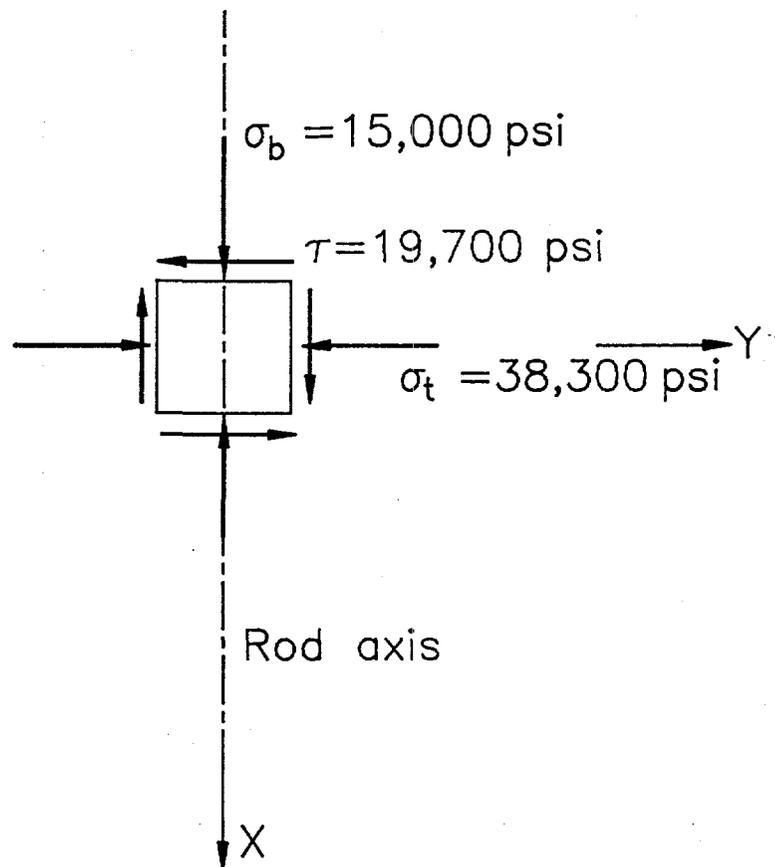
Figure 13. State of stress at the joint.
