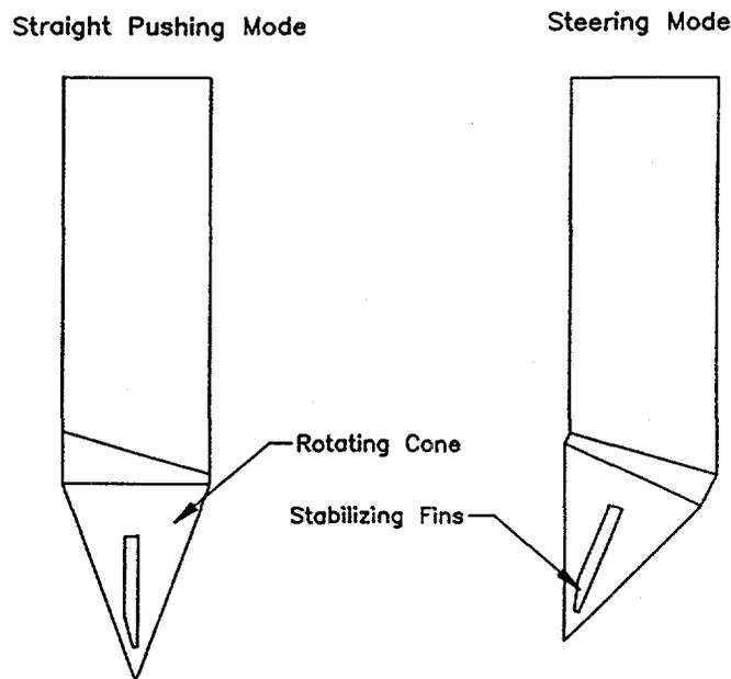
Figure 1. Modes of operation of the steering tip.
