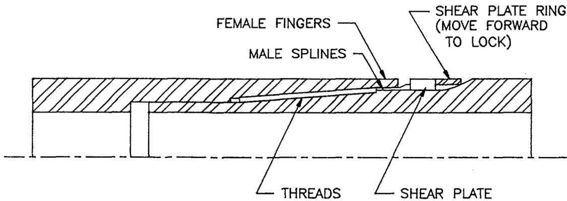
Figure 3. Assembled steerable and locking rod joint.
