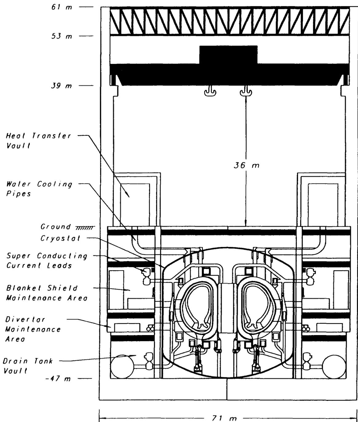
Fig. 6. Cross Section of Tokamak Building and Cryostat
