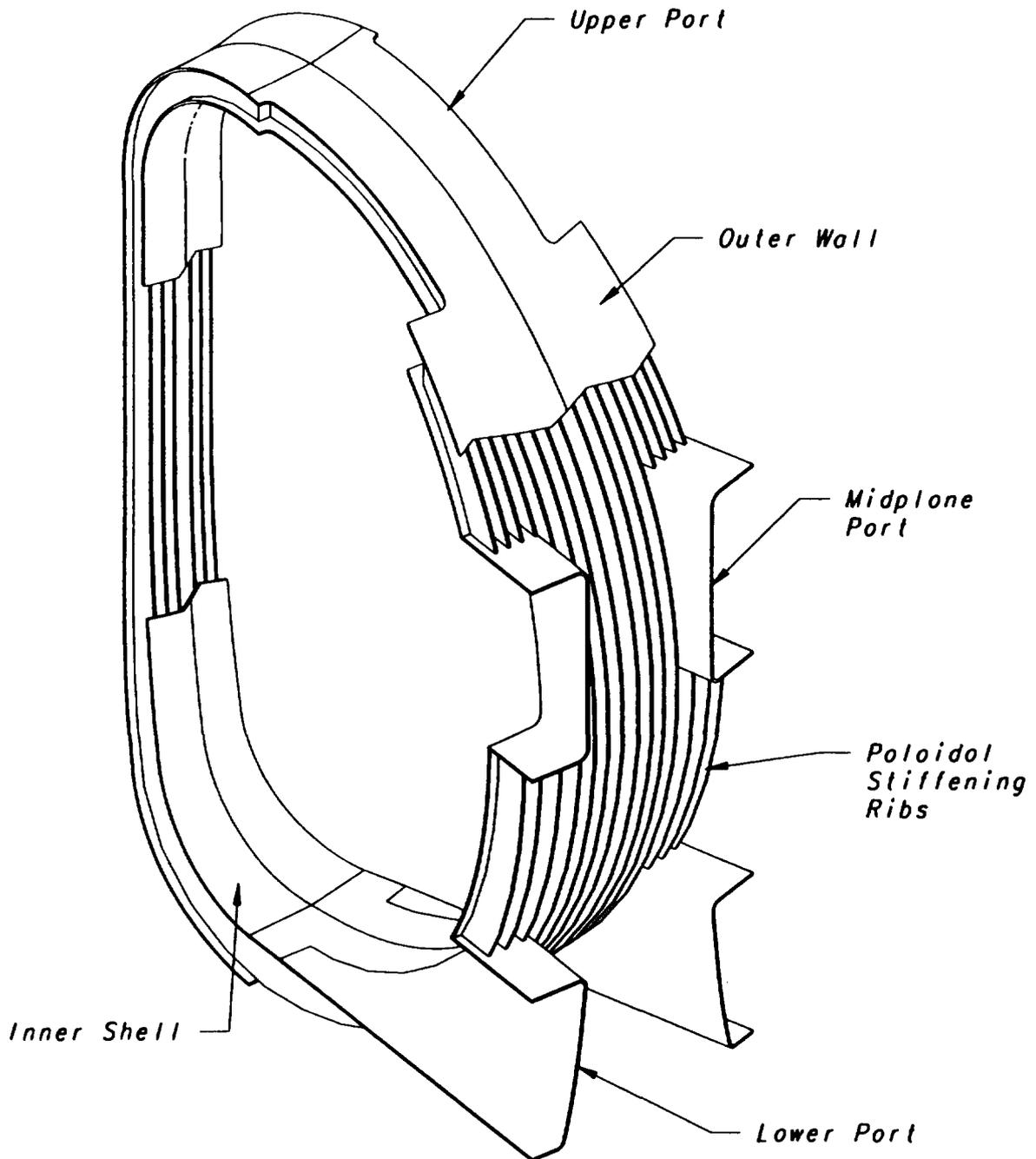
Fig. 3. Vacuum Vessel Segment
