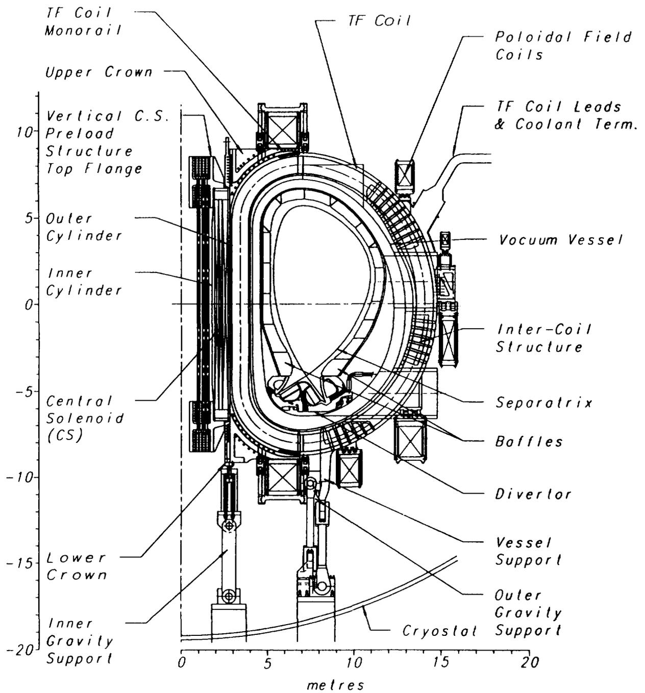
Fig. 1(a). Vertical Cross Section of ITER
