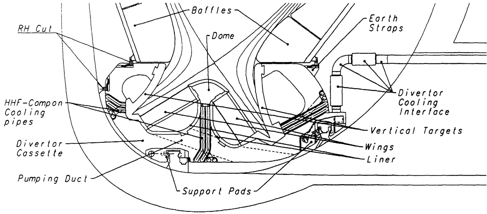
Fig. 5. Divertor Cross Section
