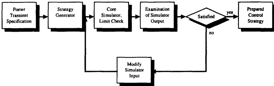
Figure 2 Procedure for predictive simulation with SCORPIO
