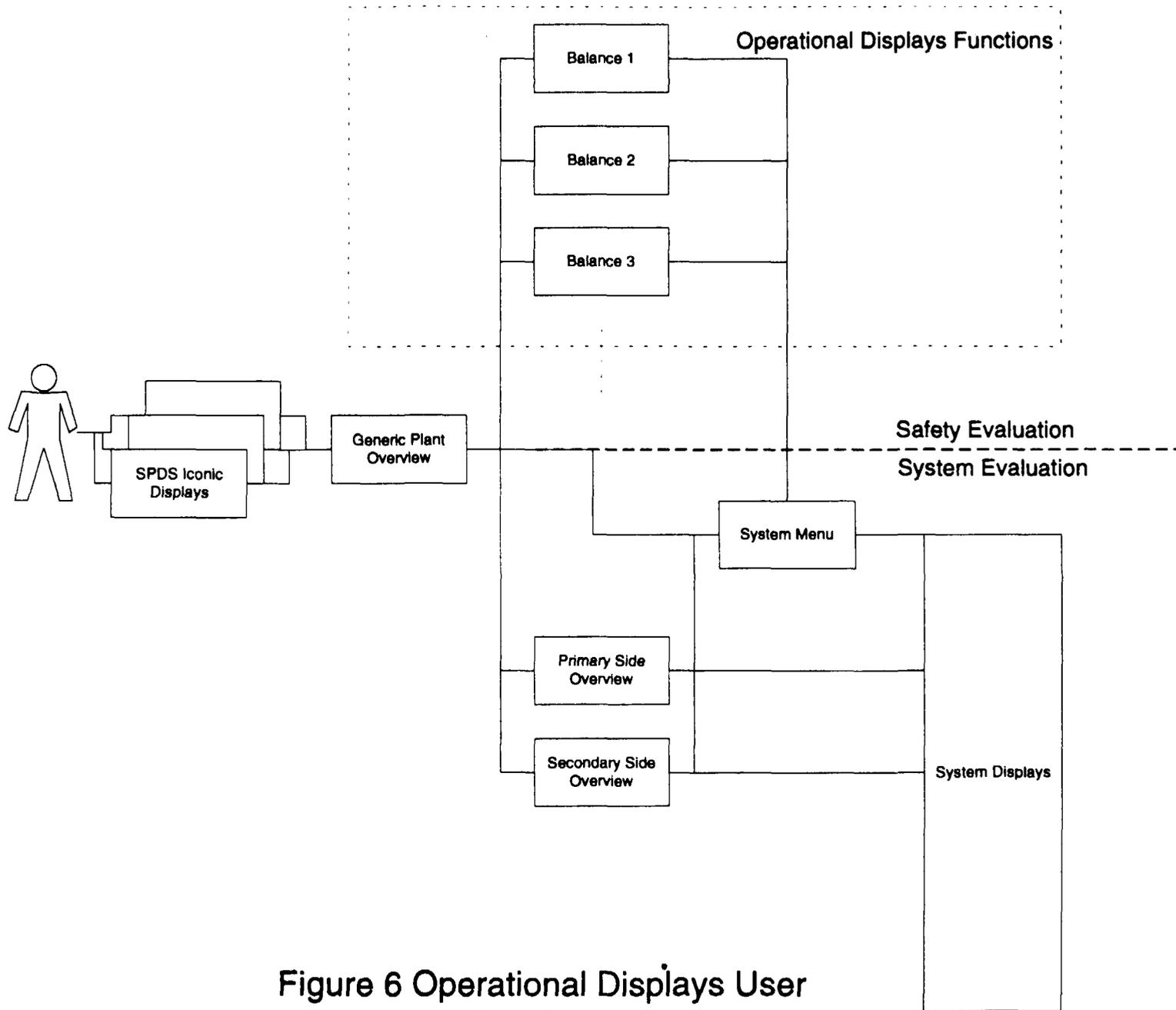
Figure 6 Operational Displays User Interface
