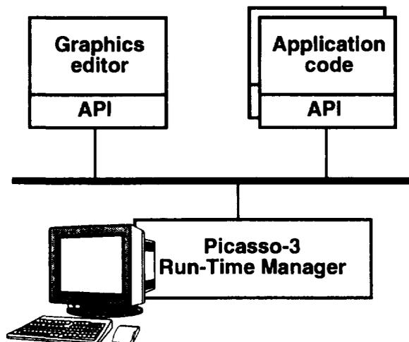
Figure 1. The end-user interacts with the user interface realised by the RTM. Application programs, communicating through the API library, can be distributed in the network. The GED is itself an ordinary Picasso-3 application utilizing the API.
