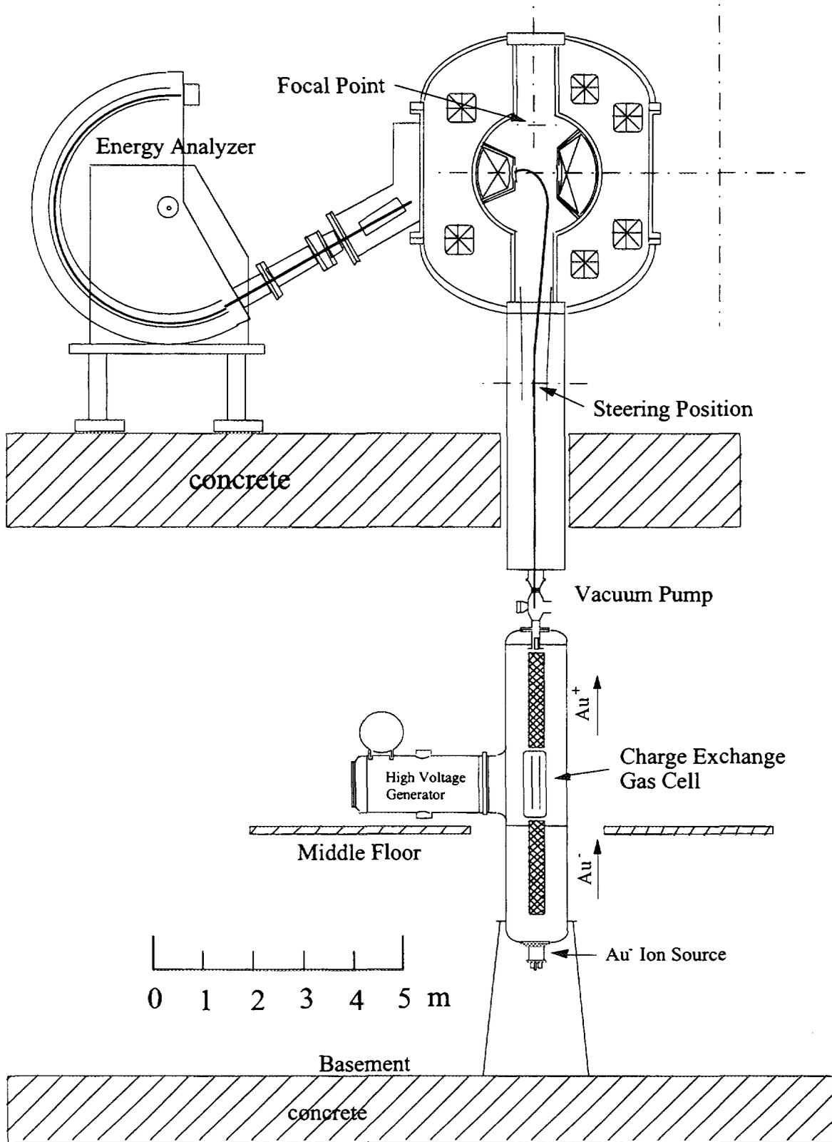
Fig. 2. A schematic drawing of the 6 MeV heavy ion beam probe.
