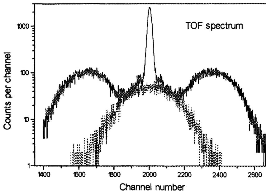
Fig. 1. Spectrum of time-of flight pseudoparameter taken for  $^{252}\text{Cf}$  source. The pseudoparameter is defined as the difference of the registration times in two selected detectors.
