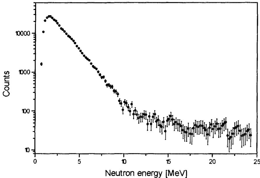
Fig.2. Fission neutron energy spectrum plotted versus laboratory neutron energy.
