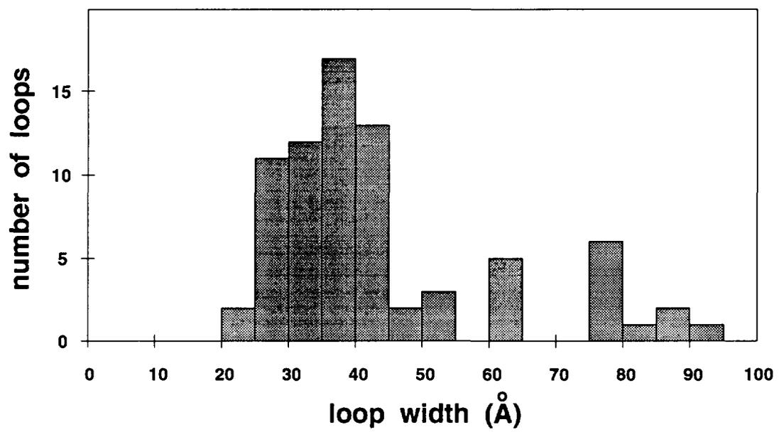
Figure 5: Histogram showing the size distribution of single loops visible on the edge of the specimen.
