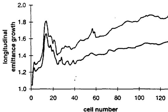
Figure 12 : Beam simulations with 5000 particles using SCHEFF with 2 different mesh sizes. Note the significant difference in emittance growth.
