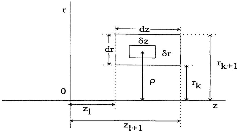
Figure 8 : Cut of the elementary ring of charge distribution in the mesh.
