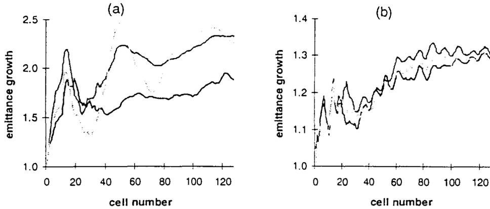
Figure 25 : Comparison of SCHERM with several ellipsoids (dark curves) to SCHERM with one ellipsoid (lighter curves) and SC3DELP (lightest curves). In (a) differences in longitudinal emittance growth occur due to the fact that the 1 ellipsoid procedure assumes a symmetrical beam. Good agreement, however, is found for the transverse emittance growth in (b).
