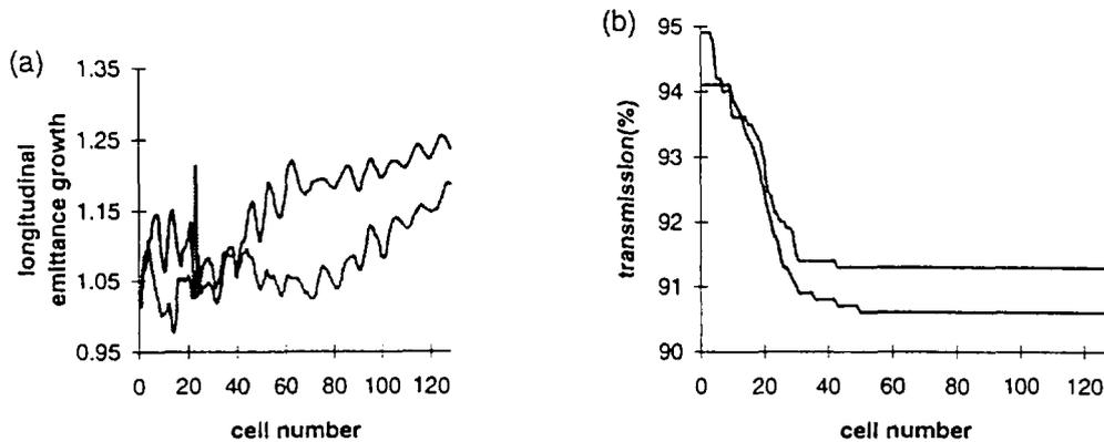
Figure 11 : SCHEFF results: In (a) the emittance growth ( i.e. current emittance divided by input emittance ) in the x-x' plane and in (b) the transmission for the CERN proton DTL (after having passed the matching section) as computed with SCHEFF for two different statistics : 1000 particles (light curves) and 5000 particles (dark curves).
