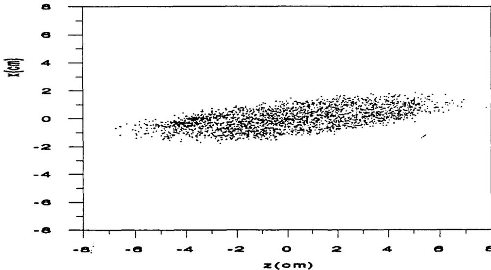
Figure 26 : A cloud of particles in the plane  $(z, x)$  for a beam crossing a bending magnet in the transport line after the CERN proton DTL.
