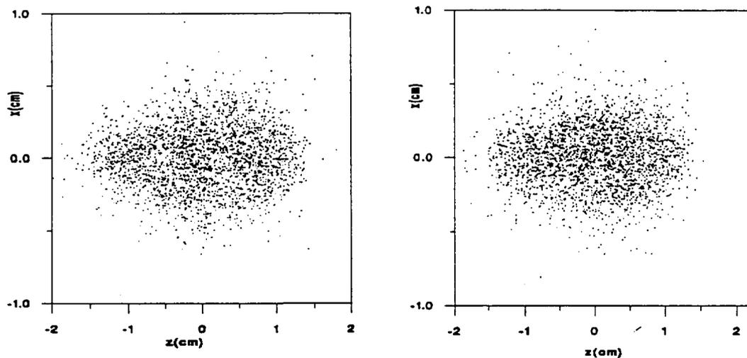
Figure 24 : In (a) are the clouds of particles at the output of the CERN proton DTL in the plane (  $z$ ,  $x$  ) for computations with SCHERM. In (b) as in (a) but for computations with the SCHEFF routine. One observes in (a) the presence of two clusters of particles, justifying the use of two ellipsoids. It is not clearly seen in (b).
