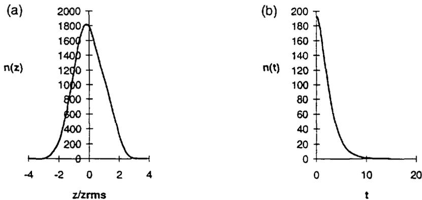
Figure 15 : In (a) the (symmetrical) real macroparticle distribution in the longitudinal direction and in (b) the computed macroparticle charge density  $n(t)$ .
