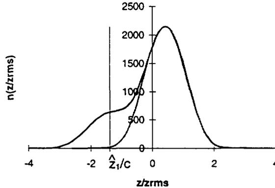
Figure 4 : The original longitudinal beam density distribution and the one of the main ellipsoid corresponding to  $m_1(v)$ .
