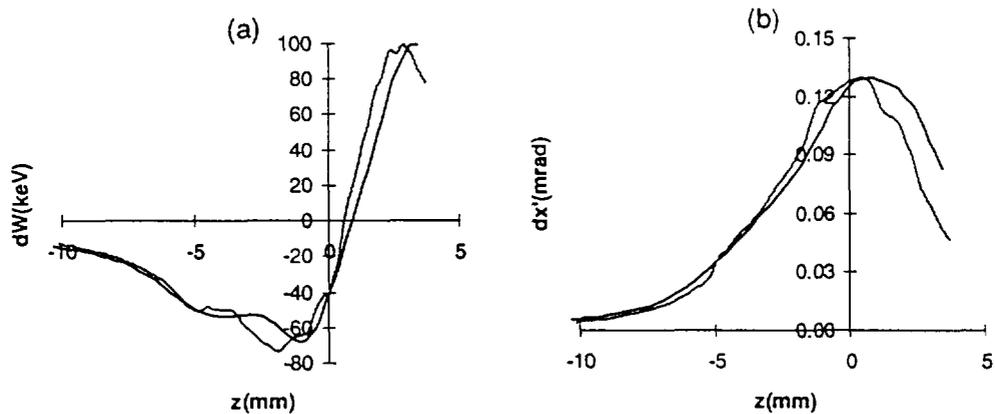
Figure 22 : Comparisons for the interdigital H structure at CERN of the impulses applied along the  $z$  direction as in fig.21.
