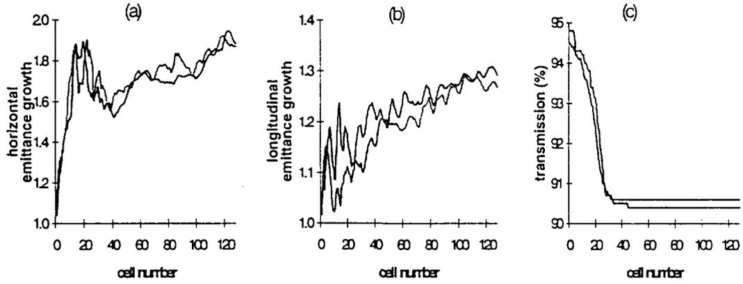
Figure 16 : The emittance growth in the horizontal (a) and longitudinal plane (b) as well as the transmission (c) as computed by SCHERM for the CERN proton linac for 2 different statistics : 1000 particles (light curve) and 5000 particles (dark curve).
