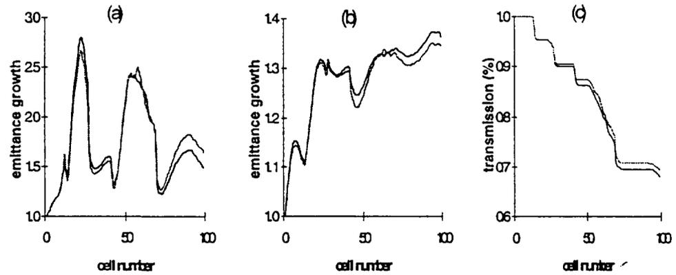
Figure 20 : Comparisons of emittance growth and of beam transmission for the interdigital H structure at CERN for acceleration of  $Pb^{27+}$ . (a),(b) and (c) are as in fig.19.
