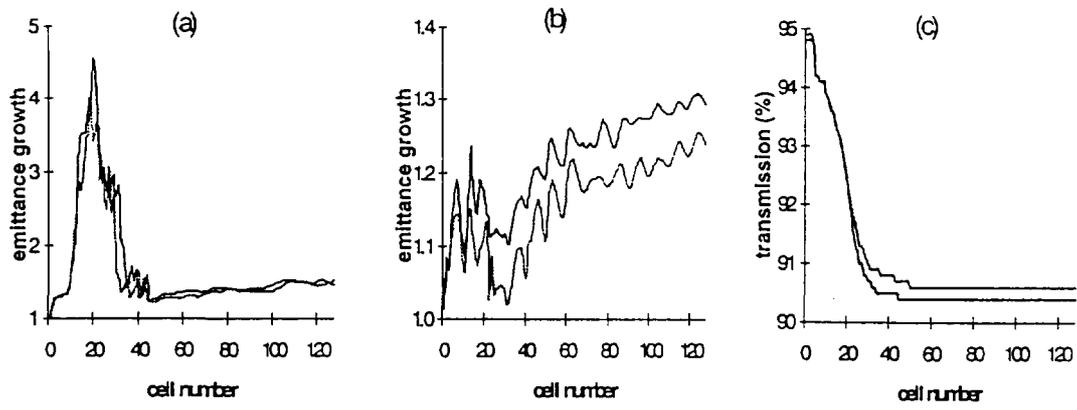
Figure 19 : Comparisons of emittance growth and beam transmission in the CERN proton DTL using SCHERM (dark curves) and SCHEFF (light curves). In (a) the longitudinal emittance growth and in (b) the horizontal emittance growth. In (c) the beam transmission is shown.
