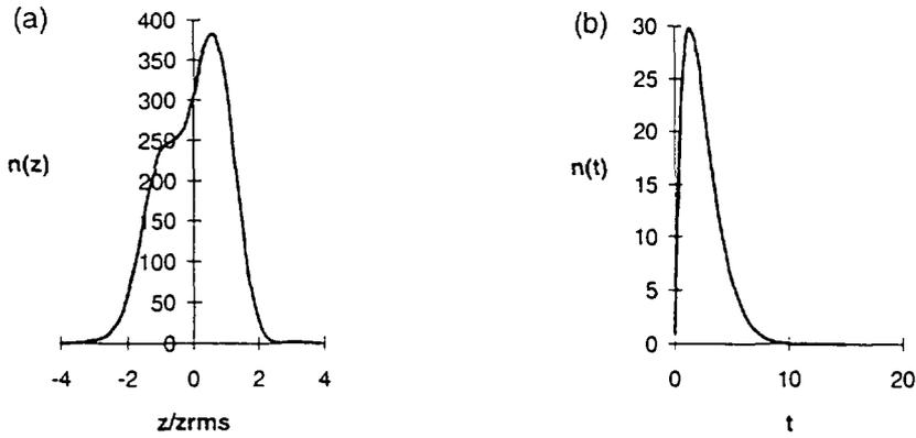
Figure 14 : In (a) a (asymmetrical) real macroparticle distribution in the longitudinal direction and in (b) the computed macroparticle charge density  $n(t)$  (in the computation the longitudinal density distribution was assumed symmetrical).
