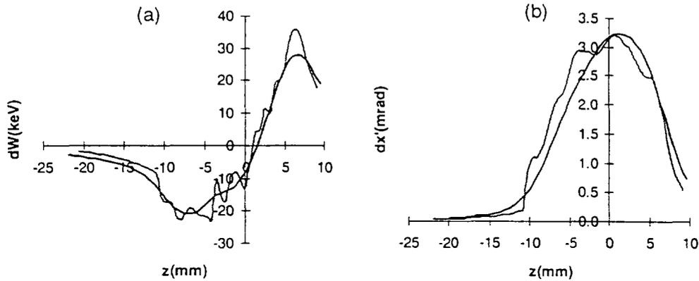
Figure 21 : In (a) comparisons for the CERN proton DTL of the impulses  $dW$  ( keV ) applied along the  $z$  direction for  $x=y=0$ . The dark curve represents SCHERM computations, the light curve the ones of the SCHEFF routine. In (b) as in (a), but for the impulses  $dx'$  ( mrad ) for  $x=0.8*a$  (  $a$  is the  $x$ -r.m.s. dimension of the bunch ) and  $y=0$ . One remarks the erratic variations obtained with SCHEFF computations as a consequence of the interpolation from node to node.
