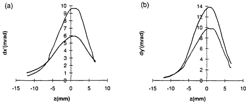
Figure 13 : In (a) the applied impulse  $dx'$  as a function of  $z$  for the position  $x = 2a$  and  $y = 0$  ; in (b) the applied impulse  $dy'$  as a function of  $z$  for the position  $x = 0$  and  $y = 2b$ . Both impulses are at the middle of a quadrupole in the matching line between the proton RFQ and linac at CERN, where  $b/a = 3.77$ .
