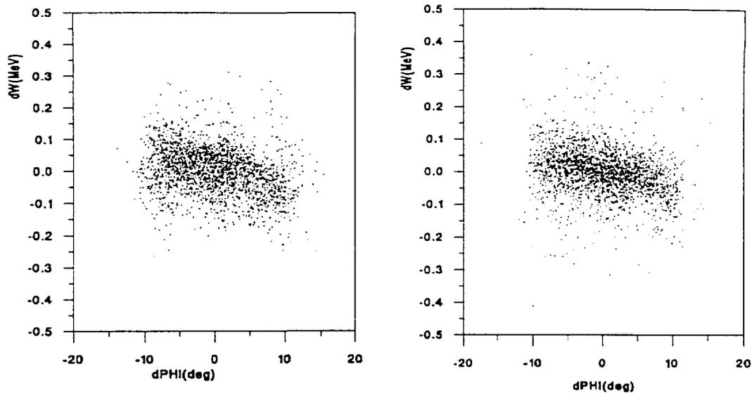
Figure 23 : In (a) the clouds of particles at the output of the CERN proton DTL in the phase space (  $dPHI$ ,  $dW$  ) for computations with SCHERM. In (b) as in (a) but for computations with the SCHEFF routine
