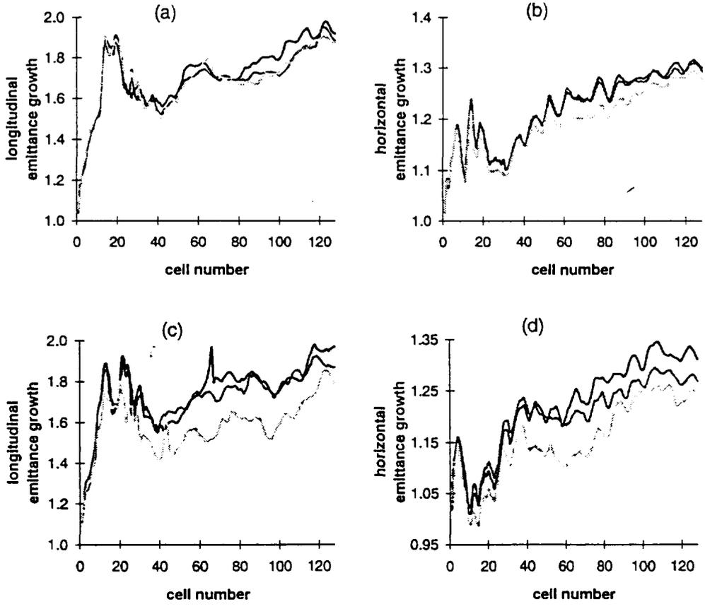
Figure 17 : In (a) and (b) the longitudinal and the horizontal emittance growth respectively, for a statistic of 5000 particles. The degrees of the Hermite polynomial in SCHERM computations are respectively 4 (light curve), 6 (darker curve) and 8 (darkest curve). (c) and (d) as (a) and (b), but with a statistic of 1000 particles.
