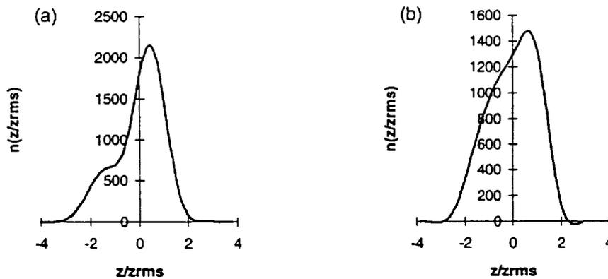
Figure 1 : The longitudinal beam density distribution  $n(z)$  for the CERN high current proton DTL [2] at 213 mA (a) and for the CERN  $Pb^{27+}$  ion interdigital H linac [3] at 10 mA (b).
