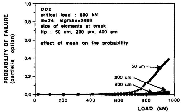
FIG 4. PROBABILITY OF FAILURE VERSUS LOAD CURVE FOR DD2 MOCK-UP. SENSITIVITY OF RESULTS TO MESH REFINEMENT
