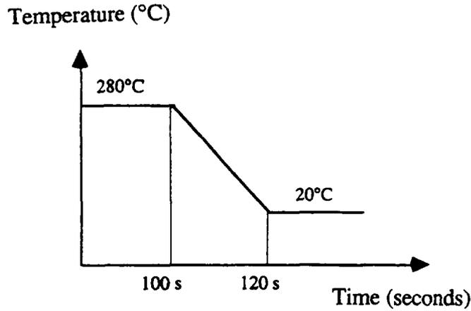
FIG 12. THERMAL TRANSIENT APPLIED TO THE VESSELS
