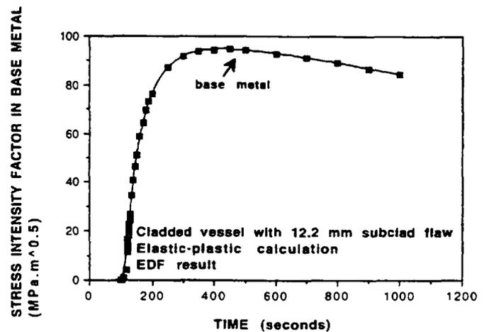
FIG 13. STRESS INTENSITY FACTOR  $K_I$  IN BASE METAL DURING THE TRANSIENT
