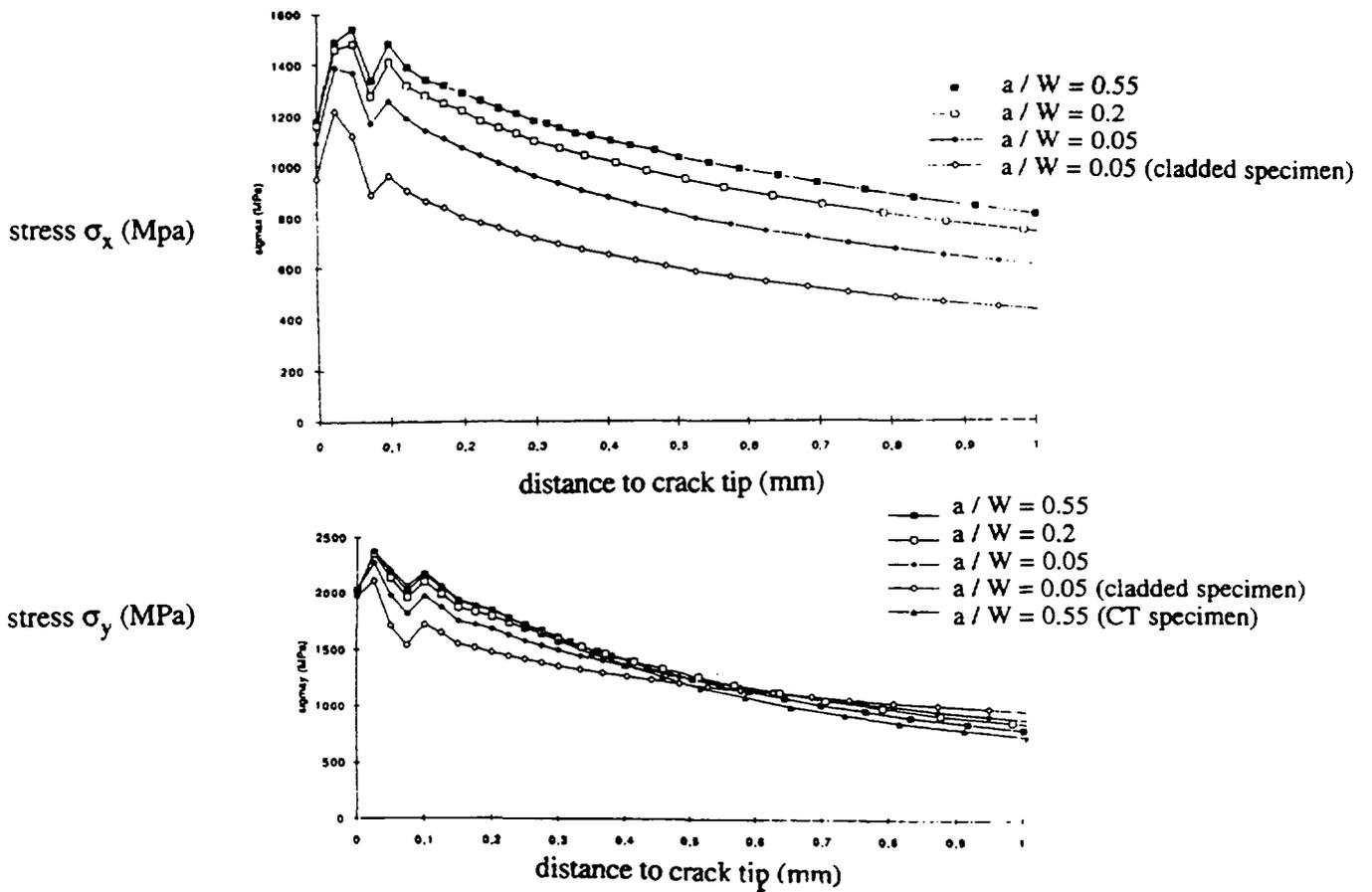
FIG 8. STRESS PROFILE ON LIGAMENT OF DIFFERENT CRACKED SPECIMENS ( $K_I = 60 \text{ MPa.m}^{0.5}$  FOR EACH SPECIMEN)
