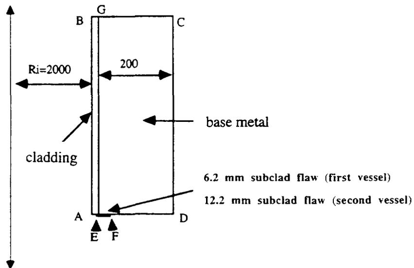
FIG 10. GEOMETRY OF THE CLADED VESSELS
