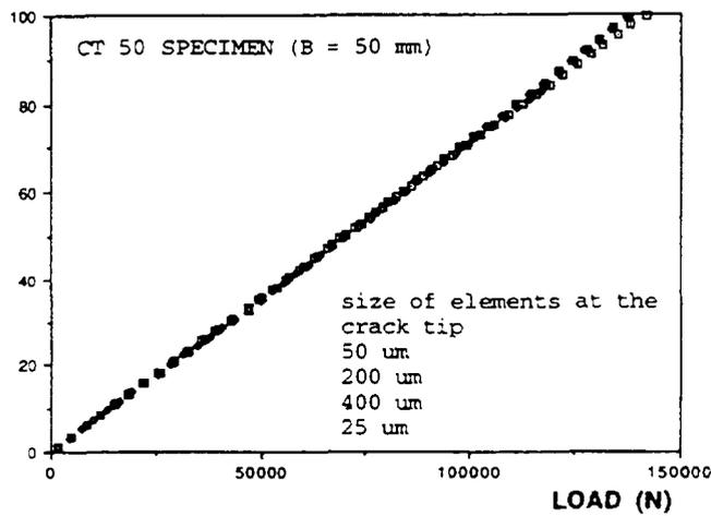
FIG 1. STRESS INTENSITY FACTOR  $K_I$  VERSUS LOAD (CT SPECIMEN)
