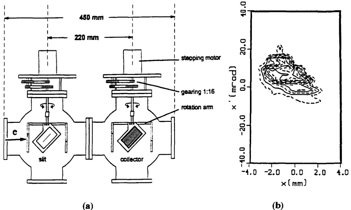
**FIGURE 3.** a) The apparatus used for the emittance measurements. The slit, on the left (0.2 mm), is scanned over the beam diameter, and for each position the angular spread is measured on the strip detector. b) A typical measurement: current 0.6  $\mu$ A, electron energy 200 eV, extraction nozzle 0.8 mm. The normalized emittance is  $\epsilon_n = 0.6 \pi$  mm mrad.
