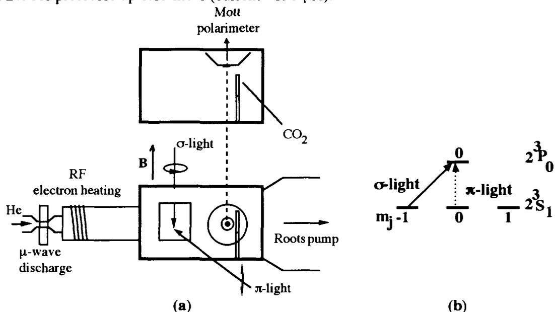
FIGURE 1. a) Schematic view of the source. b) Optical pumping scheme using He  $2^3S_1 \rightarrow 2^3P_0$  ( $D_0$ ) transition.
