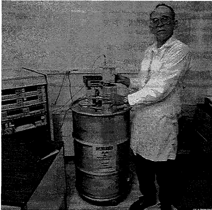
Figure 2. A sensitive, transportable calorimeter developed at Mound Laboratories. This calorimeter is currently being used for measurements of HEU and would be suitable for IAEA measurements in a nuclear facility.
