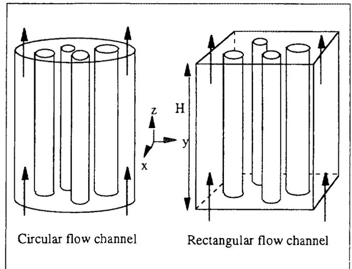
Figure 2. Circular cylinders under axial flow.
