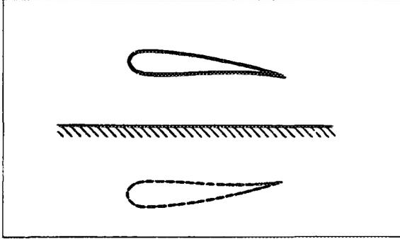
**Figure 4. Method of images applied to an airfoil in the vicinity of a wall.**
