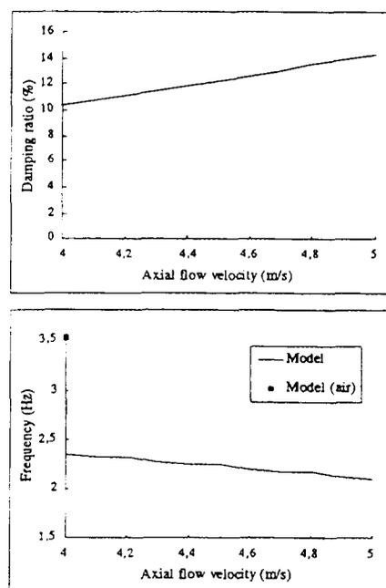
Figure 9. Evolutions of frequency and damping for the first mode of a 900MW fuel assembly.
