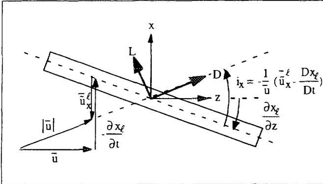
Figure 5. Flow around the cross-section of a flexible cylinder.
