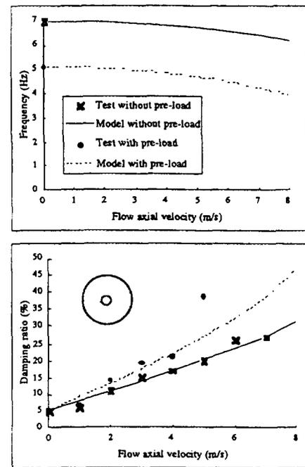
Figure 6. Evolutions of frequency and damping ratio vs. flow velocity in case A (Tanaka et al., 1988).
