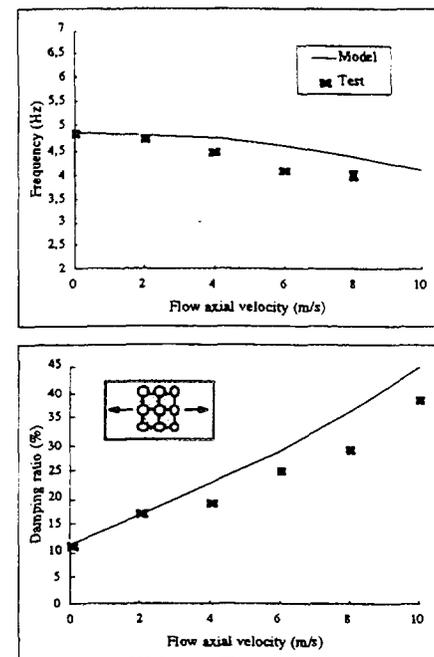
Figure 7. Evolutions of frequency and damping ratio vs. flow velocity in case B (Hotta et al., 1990).
