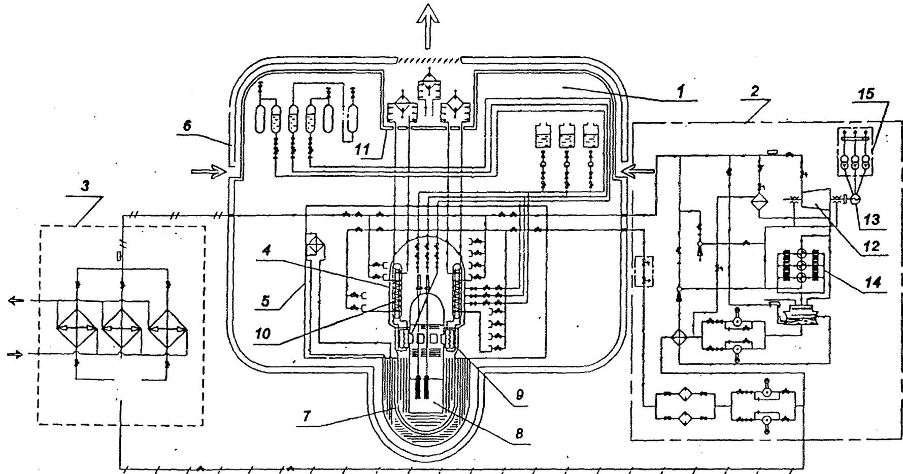
Fig.1. UNITHERM NPP Diagram
