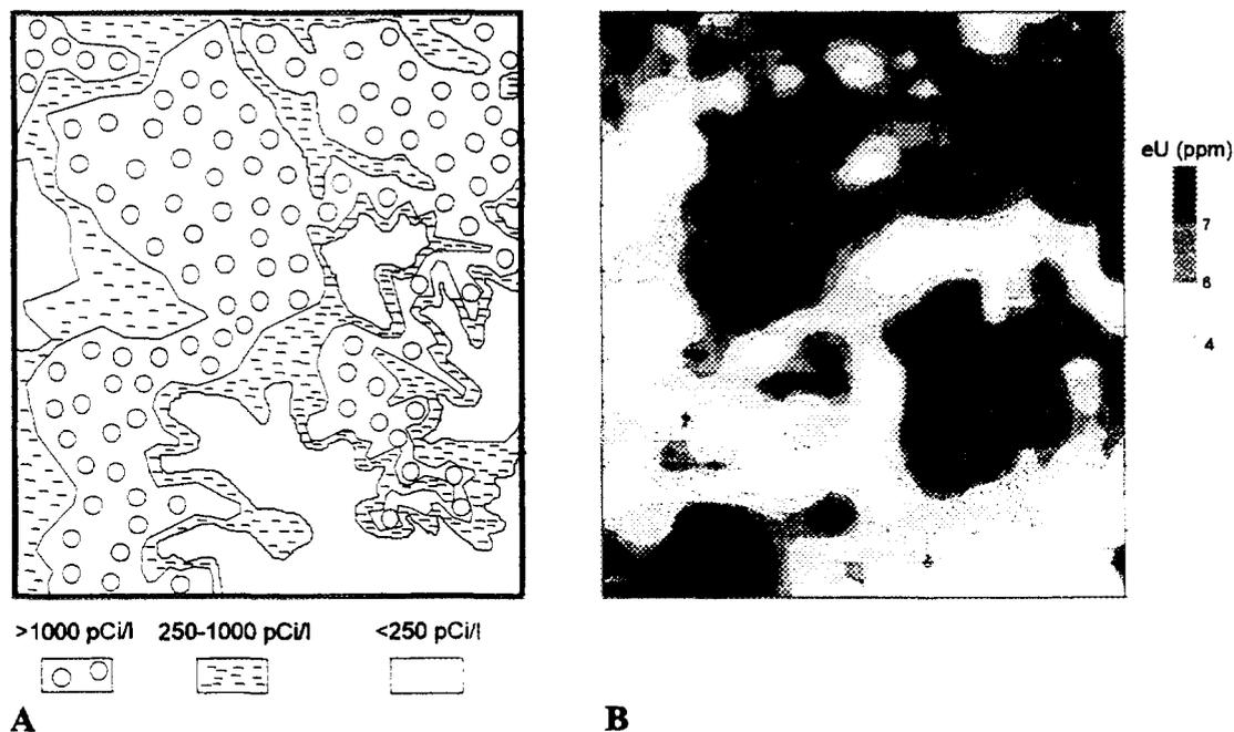
FIG. 3. Comparison between a detailed radon mapping in the vicinity of Arad, northern Negev Desert, Israel (A), and a radiometric map of the same area (B). The covered area is  $8 \times 9$  km and the original mapping scale is 1:20 000.
