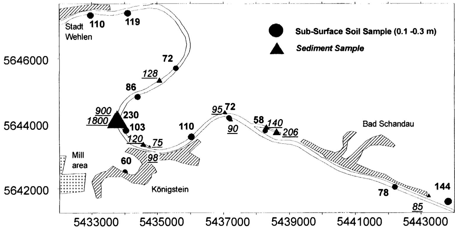
Fig. 7. Radium in soil and sediment samples (Bq/kg).
