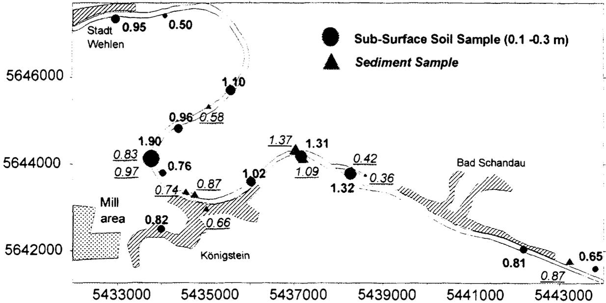
Fig. 11. U-238/Ra-226 ratios in soil (0.1-0.3 m) and sediment samples.
