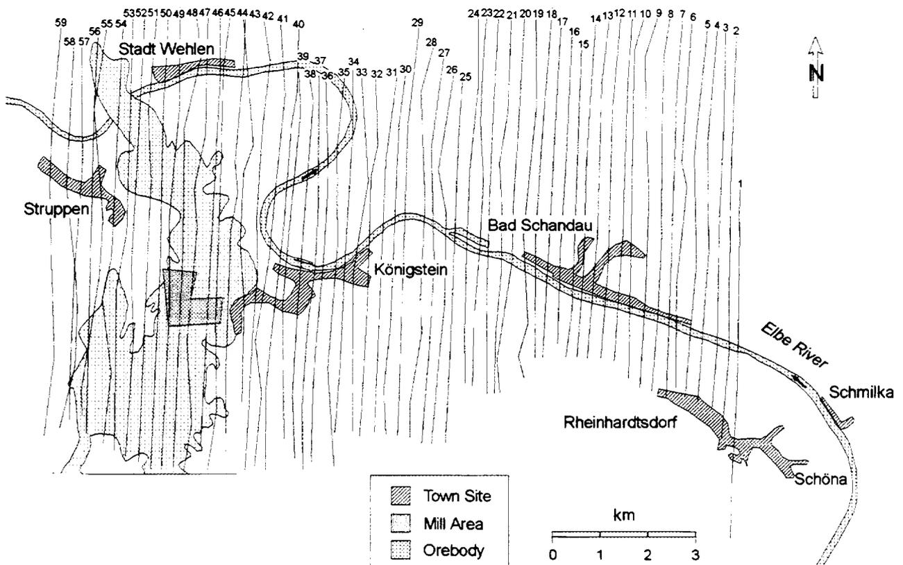
Fig. 4. Survey area - flight lines.
