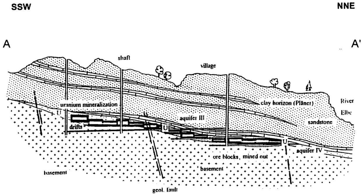
Fig. 3. Schematic cross section of the Königstein Mine.
