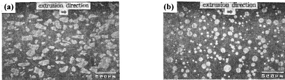
Fig. 4. The cross-sections of the U<sub>3</sub>Si fuel meat with comminuted particles (a) and atomized particles (b).
