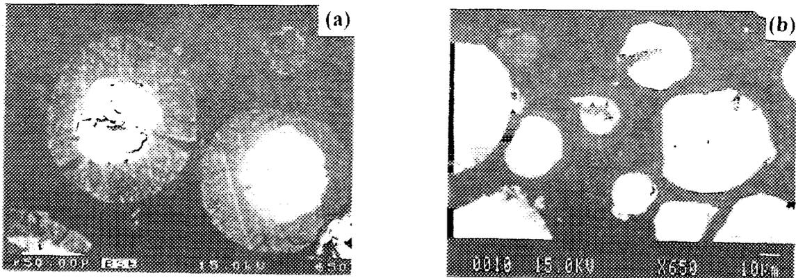
Fig. 8. Backscattered electron images of atomized fuel meat after annealing at 500°C for 20 hours; (a)  $U_3Si_2$ , (b) U-10wt.%Mo.
