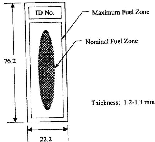
Fig. 11. The microplate.
