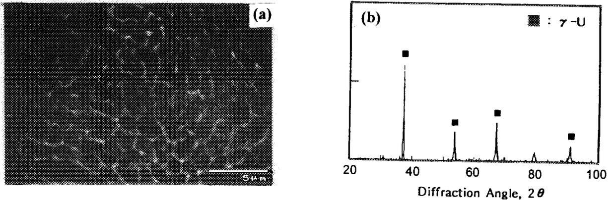
Fig. 3. The cross-sectional micrograph (a) and the X-ray diffraction pattern (b) of atomized U-10wt.%Mo alloy particles.
