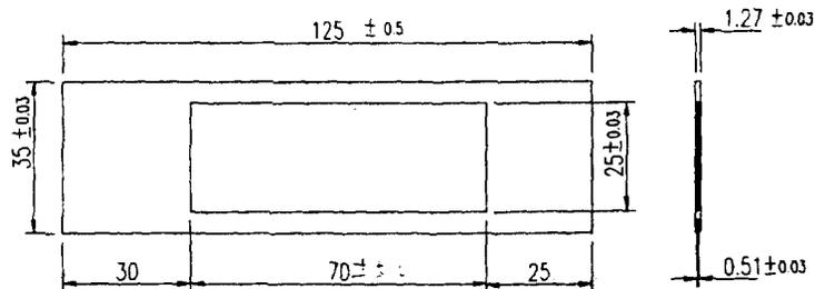
Fig. 10. An atomized  $U_3Si_2$  miniplate irradiation test rig.
