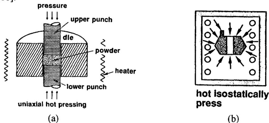
Fig. 3. The schematic showing of consolidation method of blended powders in powder metallurgy process: (a) hot pressing and (b) hot isostatic pressing.
