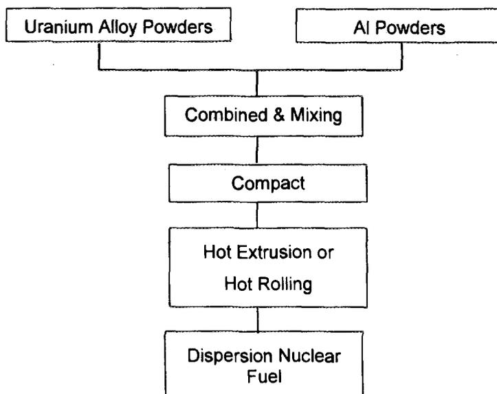
Fig. 5. Fabrication process of U/Al dispersion nuclear fuel via powder metallurgy process.
