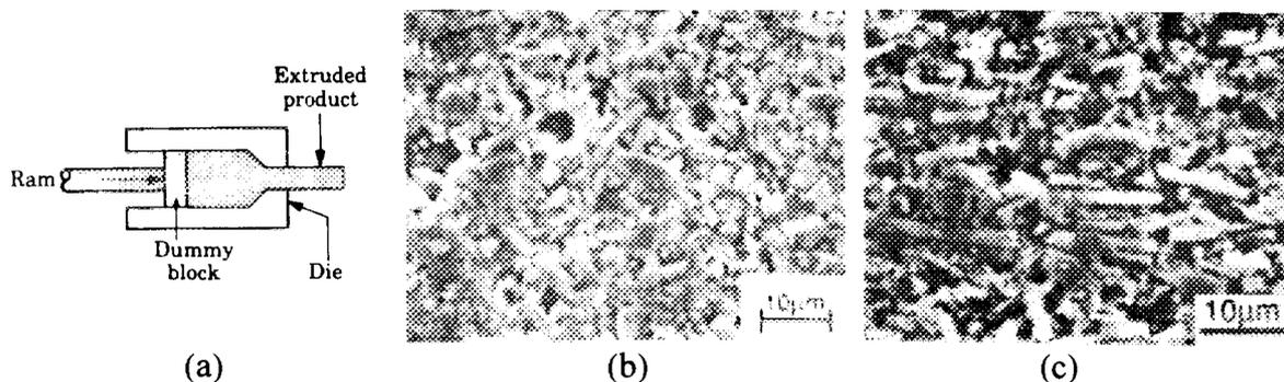
Fig. 4. (a) The extrusion process for consolidated billet. The scanning electron micrographs of SiC<sub>w</sub>/Al metal matrix composites (b) before extrusion and (c) after extrusion, showing the effect of extrusion on the aspect ratio and misorientation of whiskers in SiC<sub>w</sub>/2124Al metal matrix composites.
