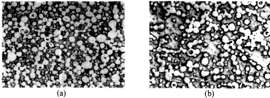
Fig. 6. (a) Typically microstructure of homogeneous by distributed  $U_3Si$  fuel particles in Al matrix and (b) microstructure of inhomogeneous by distributed  $U_3Si$  fuel particles illustrating aluminum rich area.
