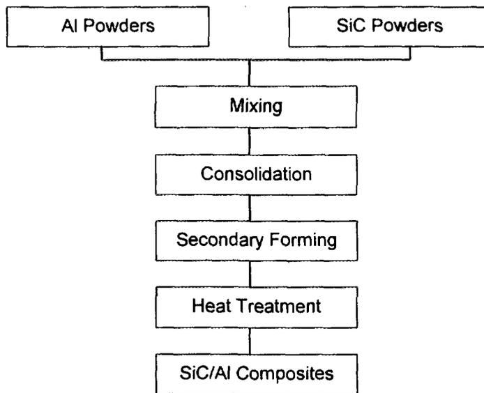
Fig. 1. Fabrication process steps of SiC/Al composites via powder metallurgy process
