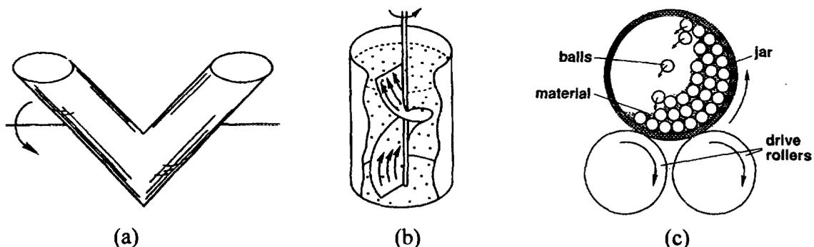
Fig. 2. The mixing methods in powder metallurgy process: (a) dry mixing, (b) wet mixing and (c) ball mill.
