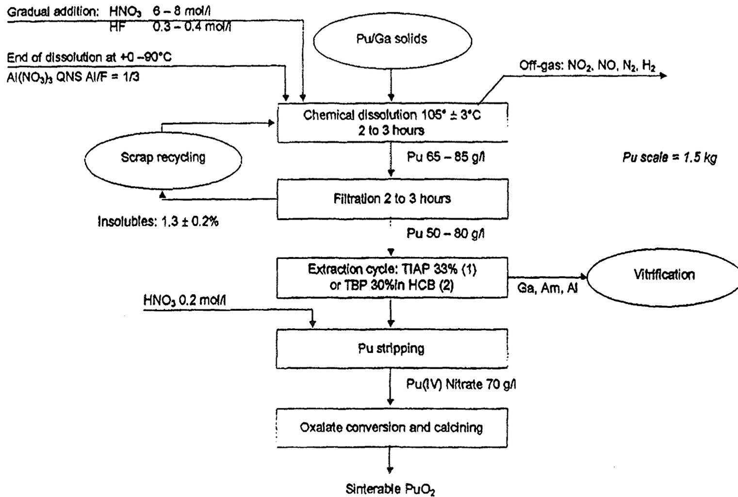
FIG. 3. AIDA/MOX reference flowsheet for converting W-Pu into  $\text{PuO}_2$
