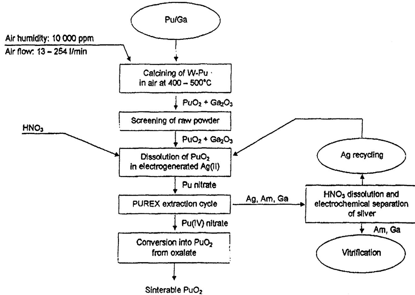
FIG. 4. Variant b of AIDA/MOX reference flowsheet: W-Pu calcining, dissolution, PUREX extraction, oxalate conversion
