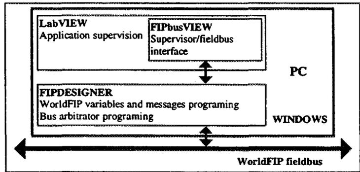
**Figure 5. Software tools for network management and supervision**
