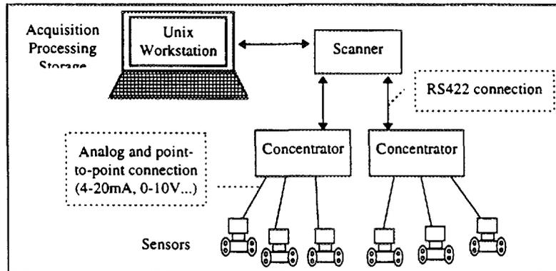
**Figure 1. Today's architecture for on-site testing in EDF power plants**
