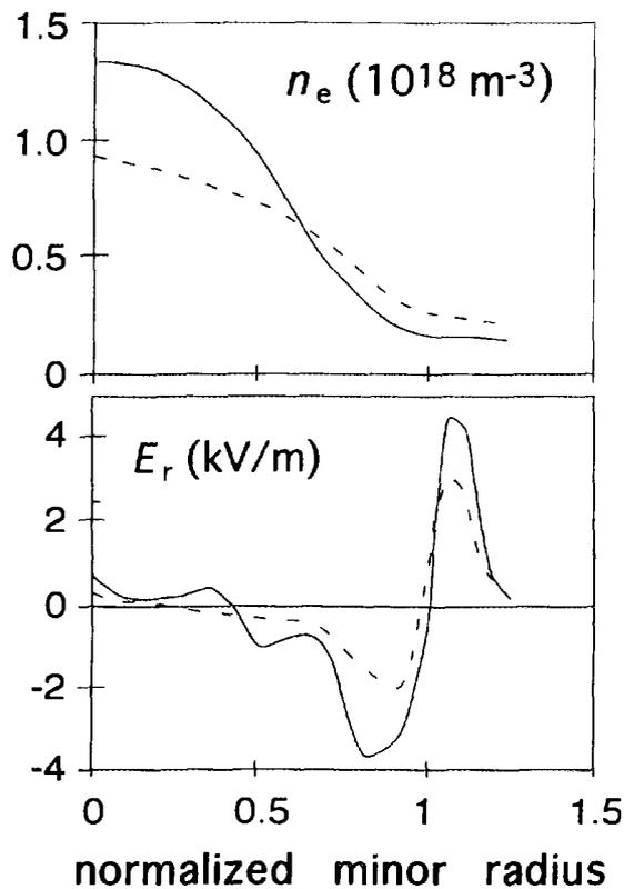
**Fig. 5.** Radial profiles of plasma density ( $n_e$ ) and radial electric field ( $E_r$ ) in H-1NF plasma. Profiles taken before (dashed) and after (solid) the transition to improved confinement.
