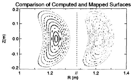
Fig. 3. Calculated and measured magnetic surfaces in the H-1NF device.
