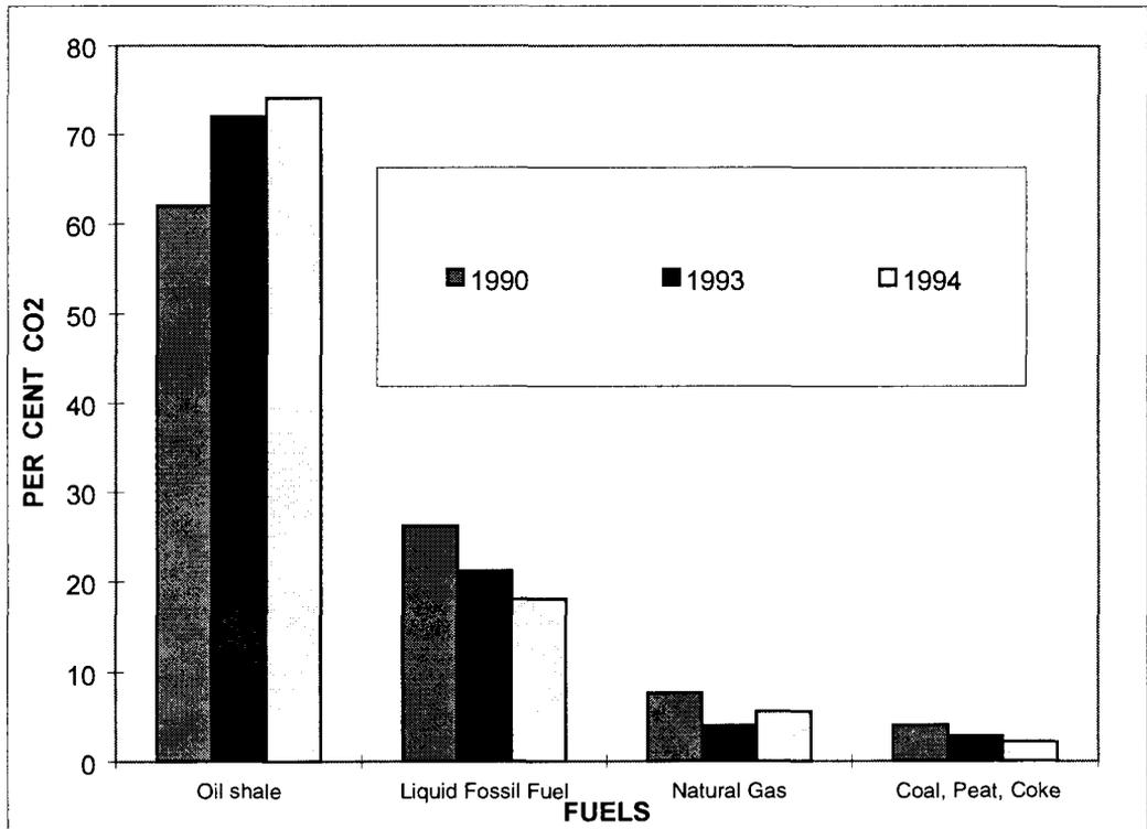
**Fig. 4.** The relative shares of CO<sub>2</sub> emissions from fuels burned in 1990, 1993 and 1994
