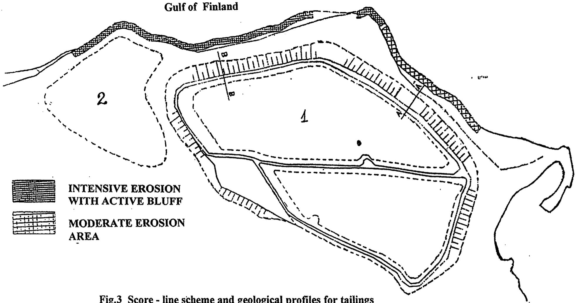
**Fig.3 Score - line scheme and geological profiles for tailings depository**
