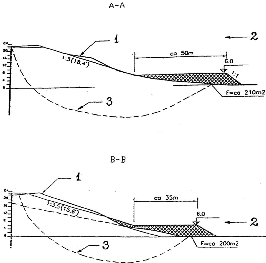
**Fig. 4. Geological cross-sections of counter balance prisms designed.**
