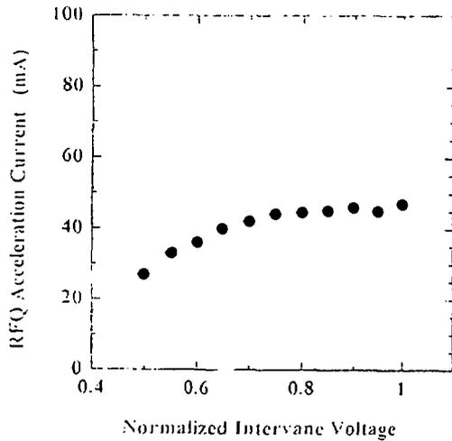
FIG. 7. Intervane voltage dependence of RFQ acceleration current.
