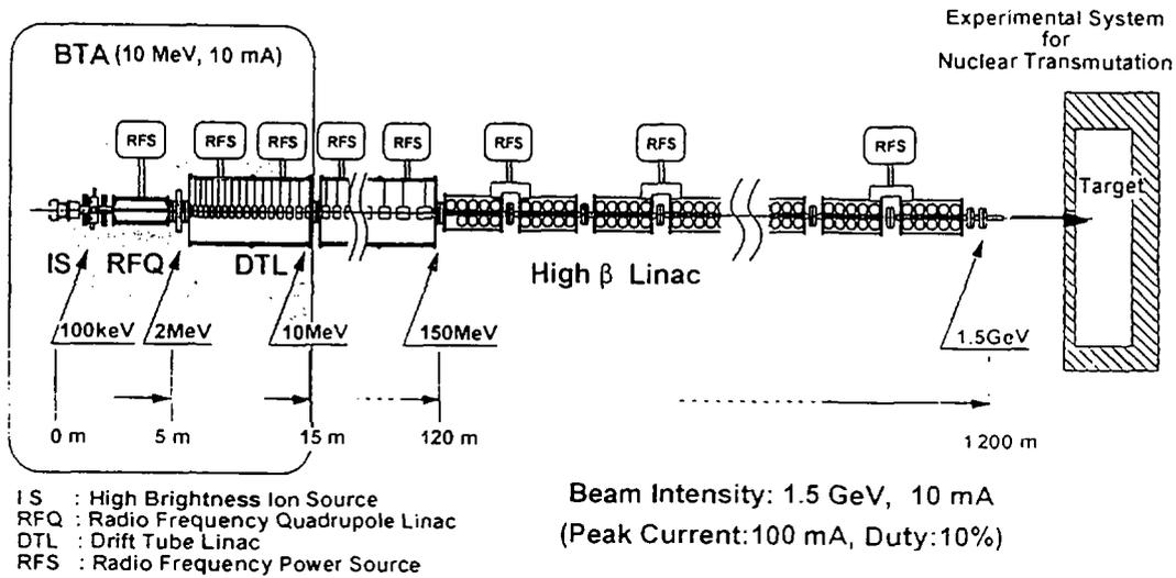
FIG. 1. A conceptual layout of the ETA
