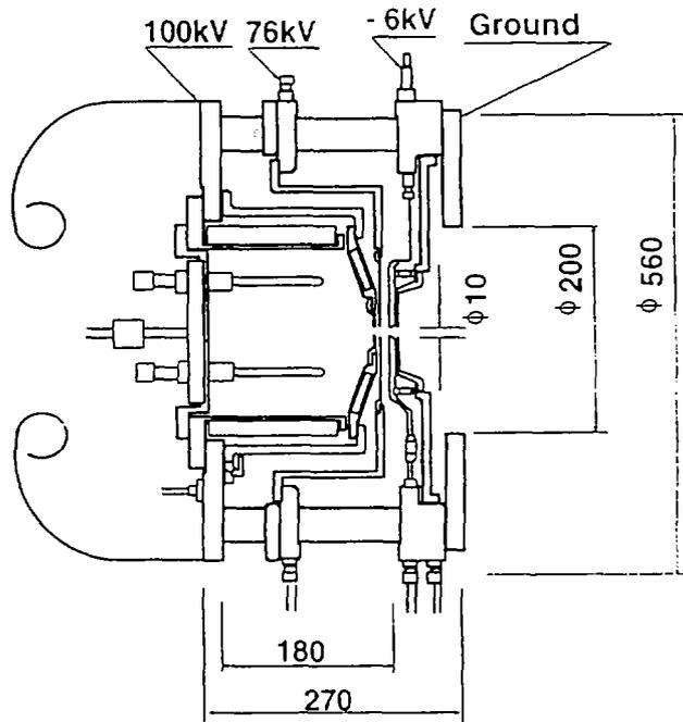
FIG. 3. A prototype of a high brightness ion source.
