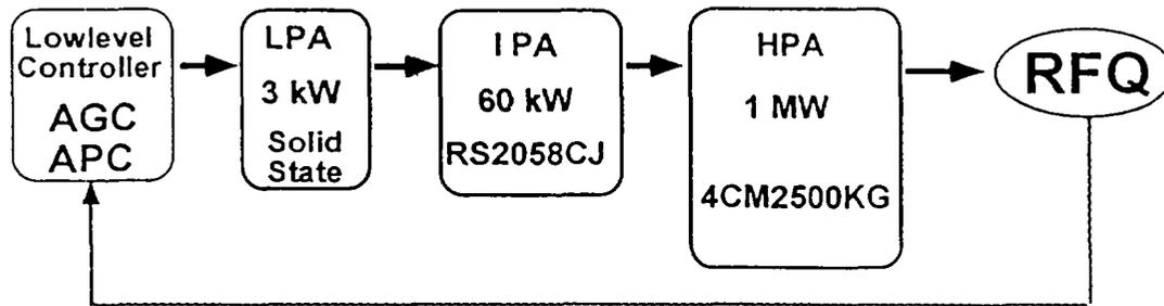
FIG. 4. A block diagram of the RF source.
