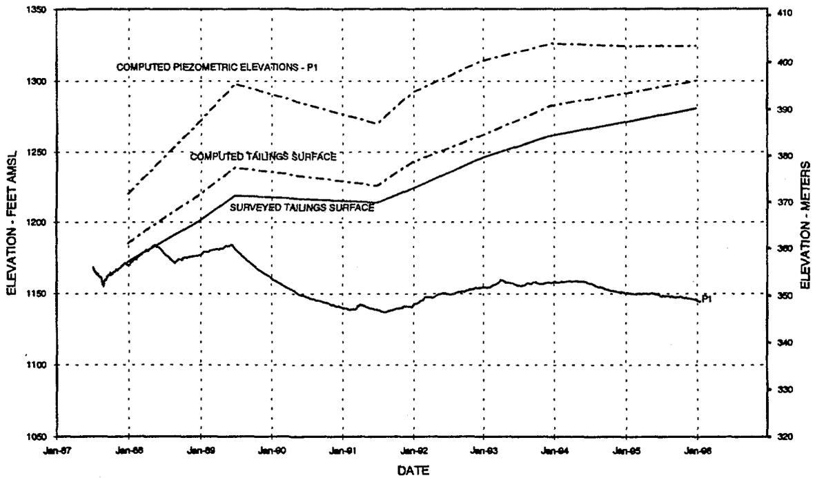
Figure 5 - RABBIT LAKE COMPUTED VS. ACTUAL PIEZOMETRIC ELEVATIONS
