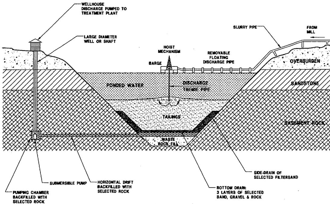
Figure 3: Deilmann Subaqueous Tailings Deposition
