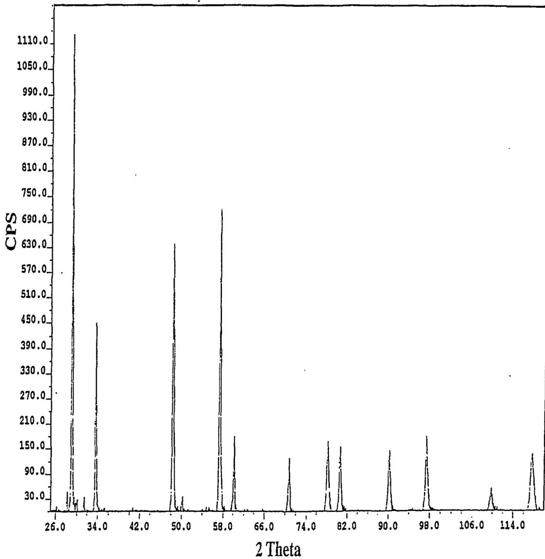
Figure 2. The XRD pattern of the pure phase zirconia with  $\text{PuO}_2$ ,  $\text{ZrO}_2$  and  $\text{Sm}_2\text{O}_3$  constituents.
