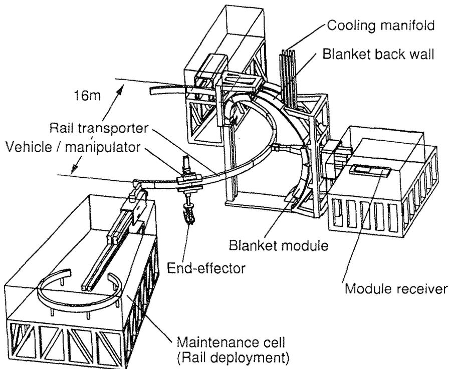
Fig. 2. Layout of the Blanket Test Platform
