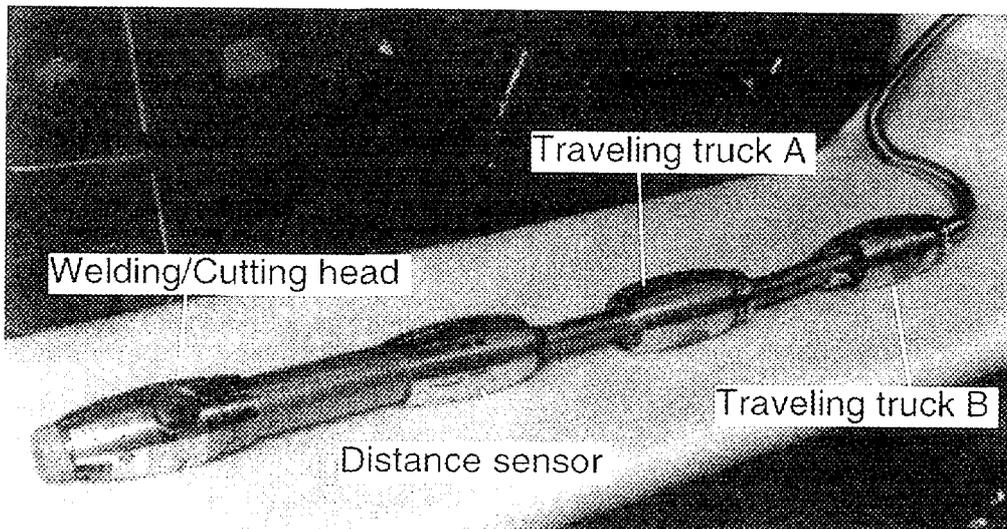
*Fig. 6. Laser based pipe welding/cutting bore tool*
