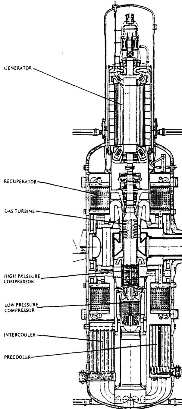
*FIG. 3. GT-MHR power conversion system incorporates US and RF technology*
