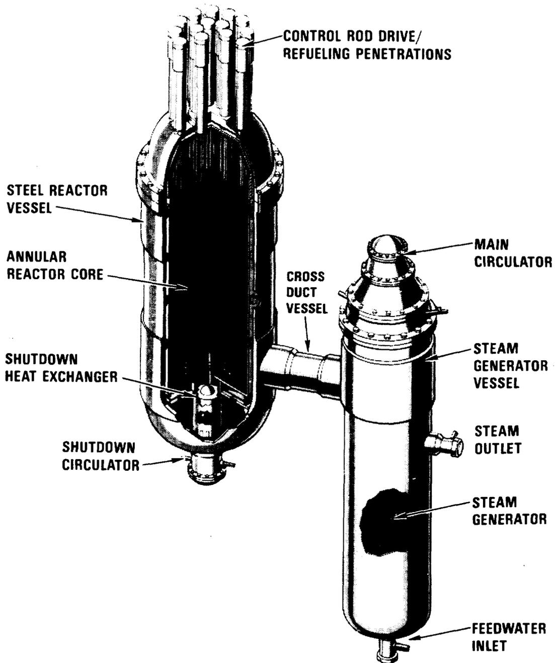
*FIG. 1. 350 MWt Modular high temperature gas reactor*
