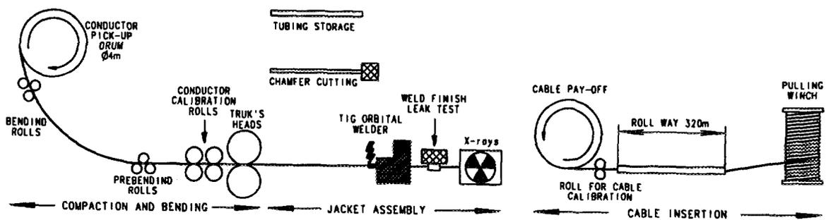
Fig. 3. Diagram of Ansaldo Jacketing Line
